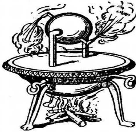
Figure 2.1: Aeolipile Developed by Hero of Alexandria(Meher-Homji, 2000)
