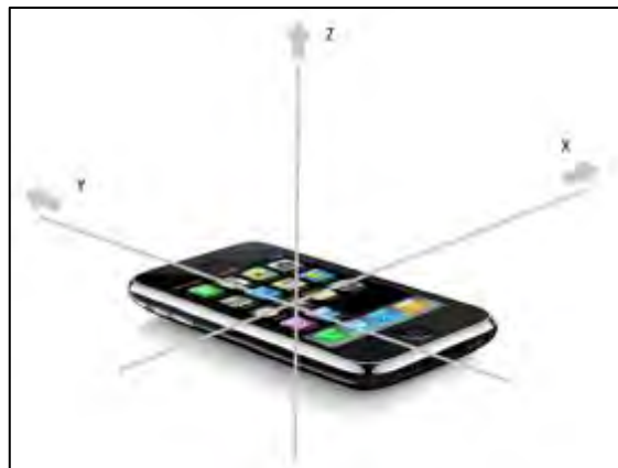
Figure 2.2: The orientation of x,y and z axis orientation based smartphone.
