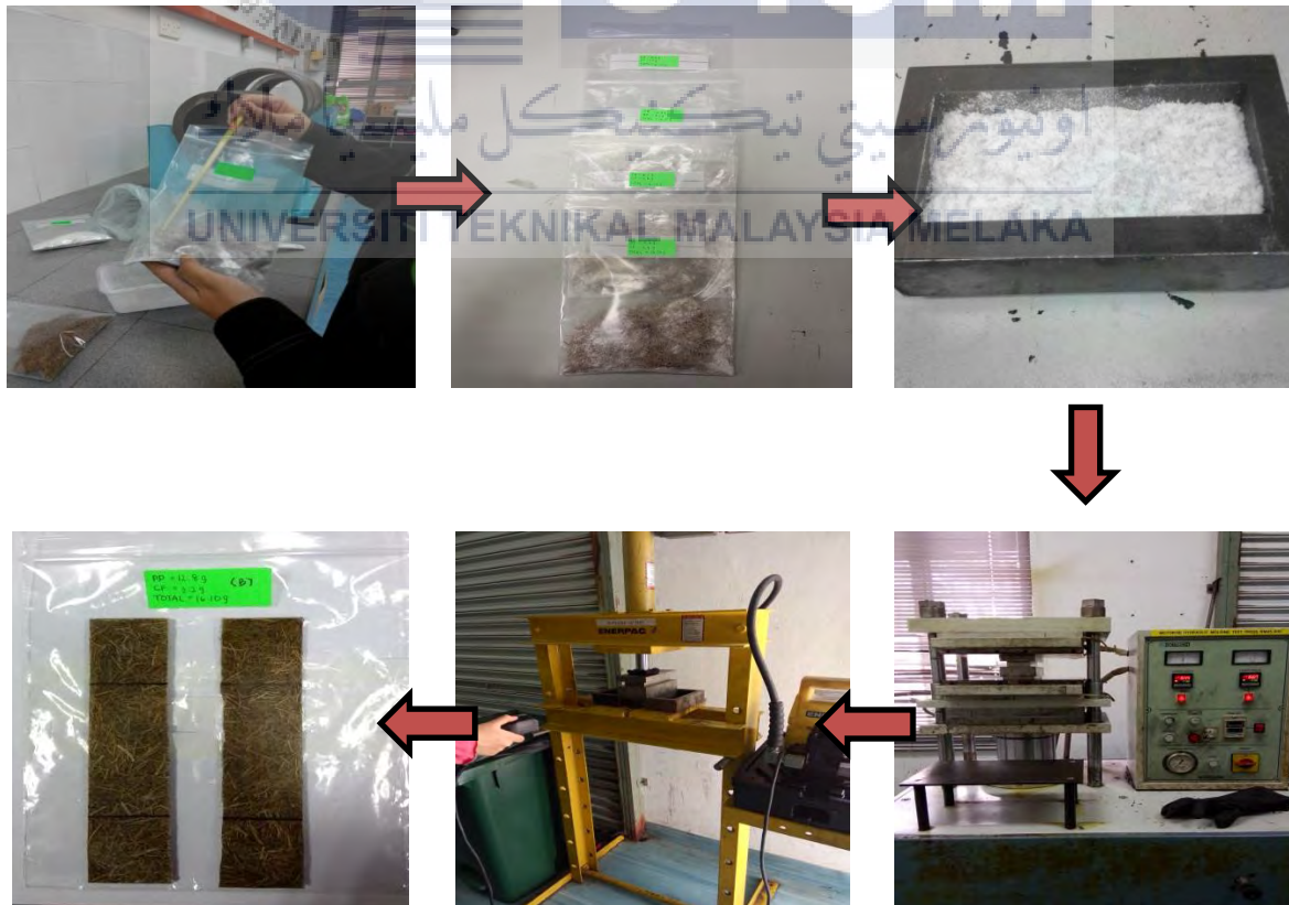
Figure 3.4: The fabrication process of composites
