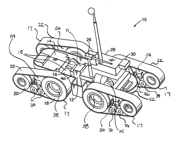
Figure 2.2 hybrid wheel and track vehicle drive system
