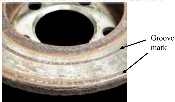
Figure 2.4: Groove marks that occur on brake disc. (Source from Meyle Product)
