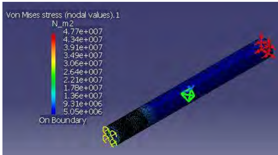
Figure 4.6b: Value of von misses stress for design concept 5.
