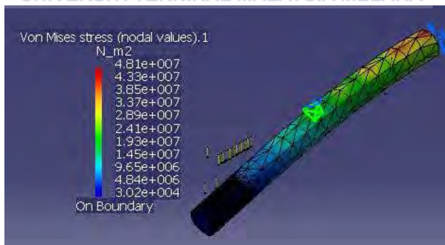
Figure 4.4b: The result from finite element analysis that shows the value of von misses stress
