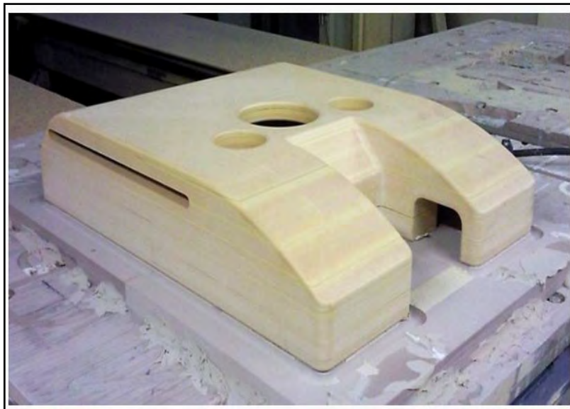
Figure 2.3: Syntactic foam block machined robot's body.
