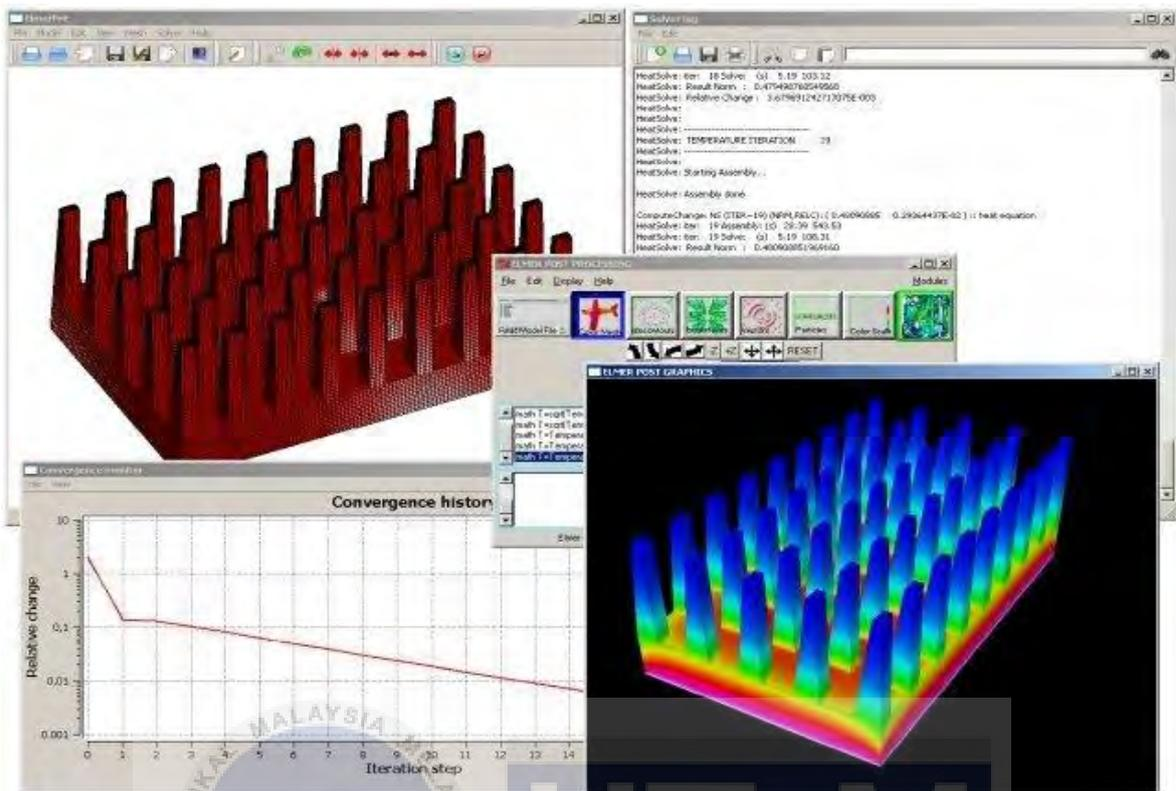
Figure 2.8: Finite Element Analysis Operation of Software 3
