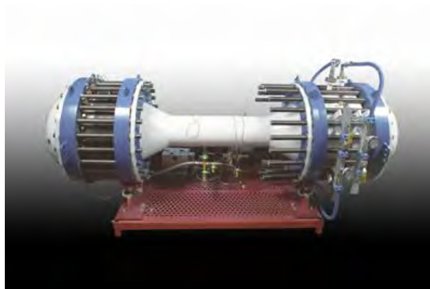
Figure 1.2 TRITON Shipboard Thermoacoustic Cooler
