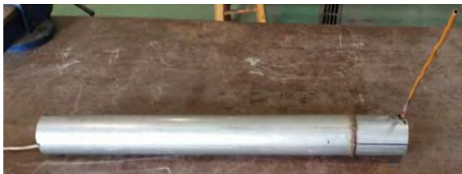
Figure 3.13: Full helical coil fit in exhaust pipe
