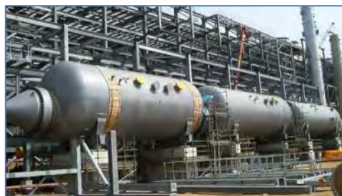
Figure 1.2: Shell and Tube Heat Exchanger in petrochemical industry
