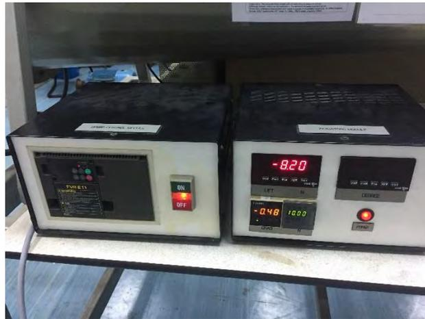
Figure 3.4: Speed Control Module and Indicator Module.
