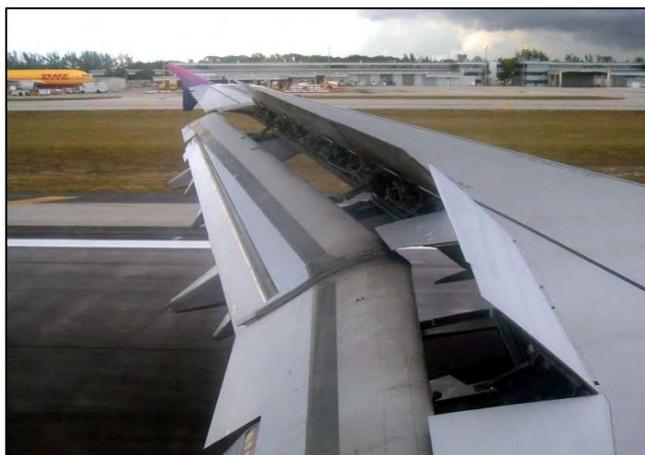
Figure 2.02: Deployed flaps and spoilers uncover VGs close to the leading edge on a flap during landing. ([https://en.wikipedia.org/wiki/Spoiler\\_\(aeronautics\)\)](https://en.wikipedia.org/wiki/Spoiler_(aeronautics))))
