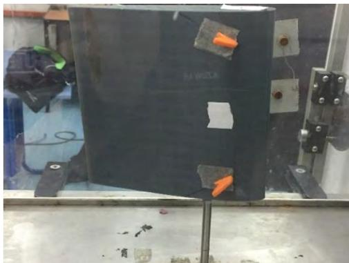
Figure 4.16: Experimental Setup for Modify Case. (Leading Fin VG)
