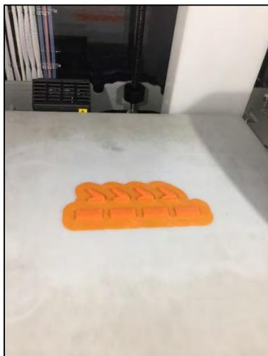
Figure 3.7: Fin and Rectangular Shaped of Vortex Generator.
