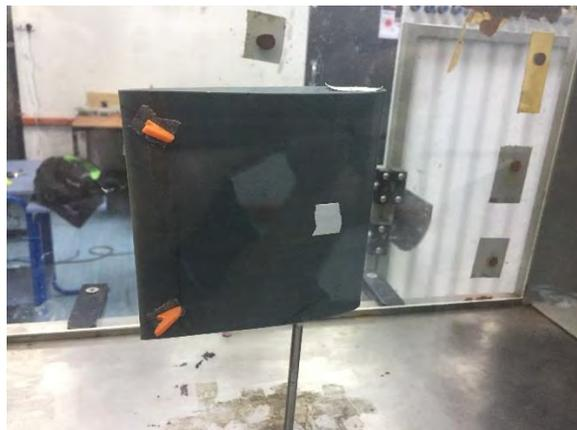
Figure 4.22: Experimental Setup for Modify Case. (Trailing Fin VG)
