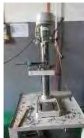
Figure 3.6: Drilling Machine
