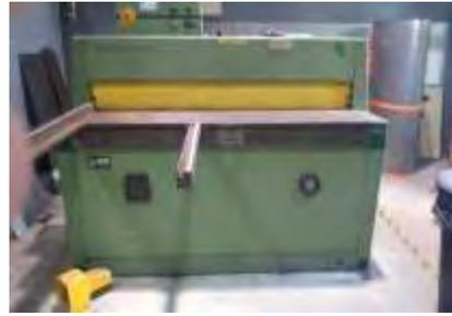
Figure 3.5: Shearing Machine
