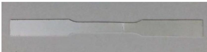
Figure 3.6: Tensile test specimen after fabrication
