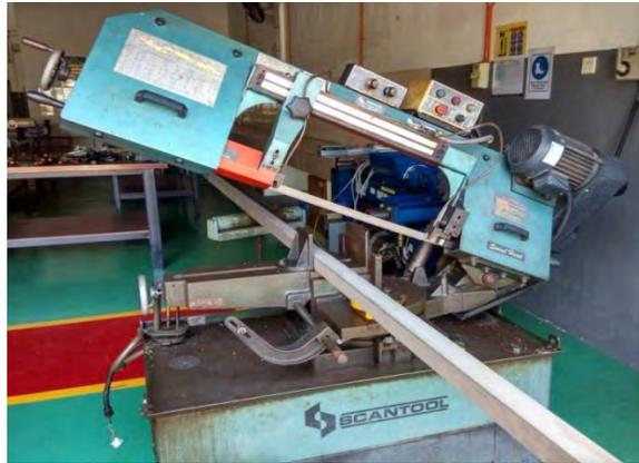
Figure 3.9: Band saw cutting machine
