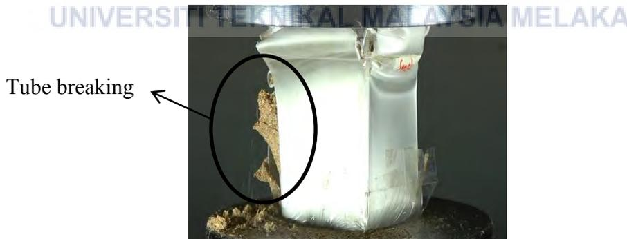
Figure 4.7: Breaking behaviour of square tube ( $L=150$  mm,  $t= 1.10$  mm,  $c= 50.6$  mm) during quasi-static axial loading
