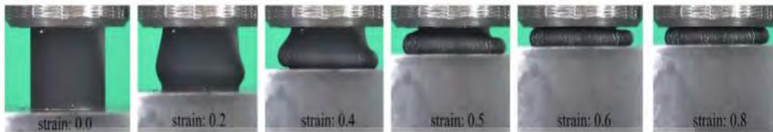
Figure 2.11: Tube structure undergoes axial compression
