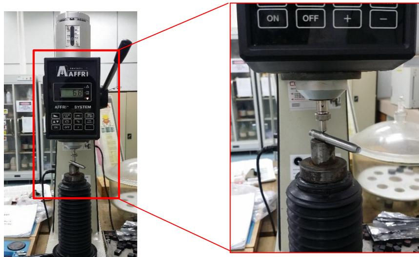
**Figure 3.7:** Setup of Hardness Test
