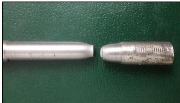
**Figure 3.5:** The Cup and Cone Fracture Behaviour of a Ductile Metal
