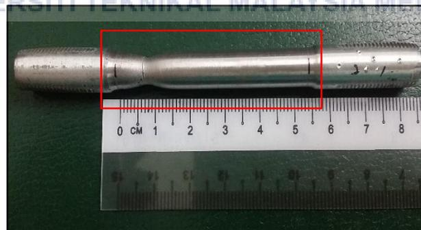
**Figure 3.3:** Gauge Length at Failure of Specimen 1
