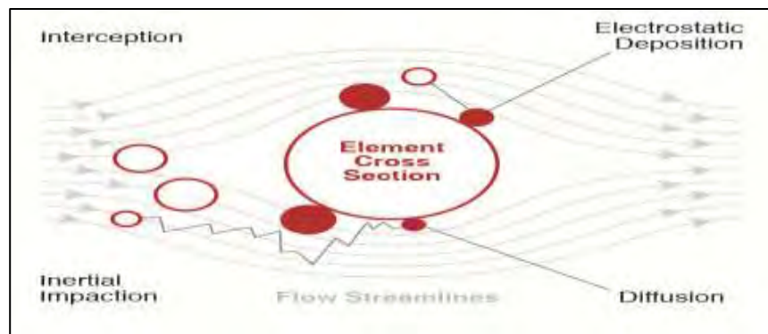
Figure 2.2: Aerosol filtration mechanism illustration (Chuanfang, 2012).
