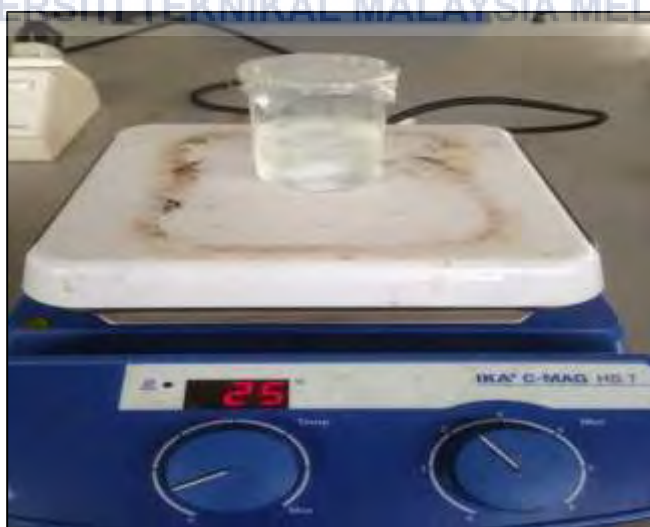
Figure 3.5: Magnetic stirrer process of PVA and H_2O solution
