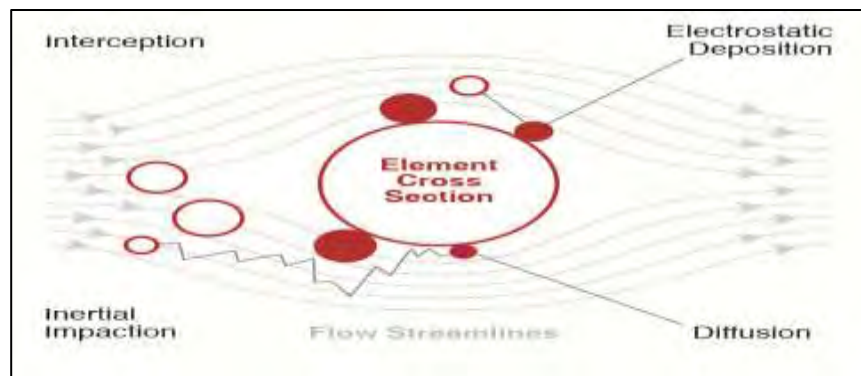
Figure 2.2: Aerosol filtration mechanism illustration (Chuanfang, 2012).
