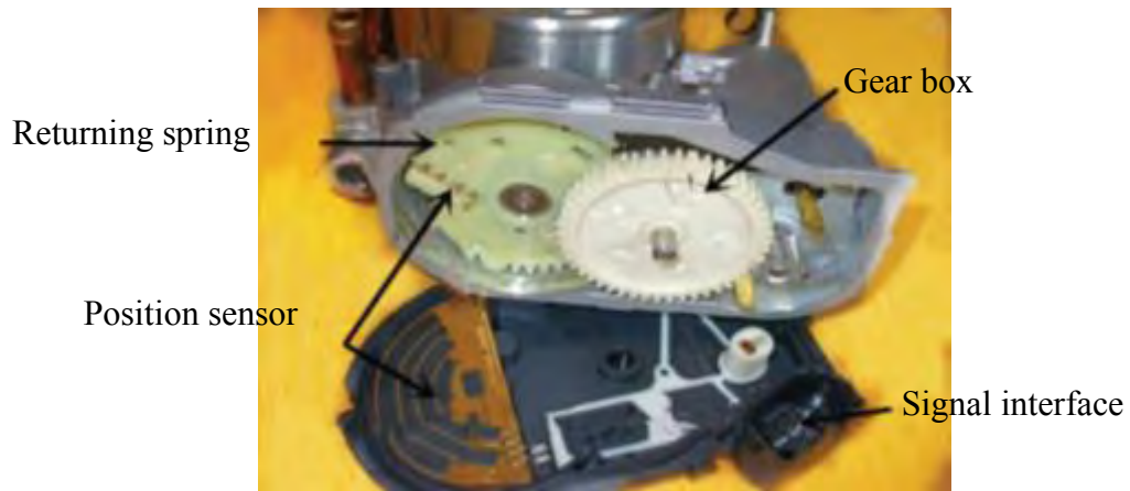
Figure 1.2: Internal view of ETB.
