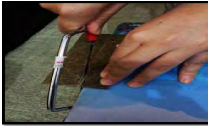
Figure 3.23: The PALF/PP composites samples were cut into specified dimension
