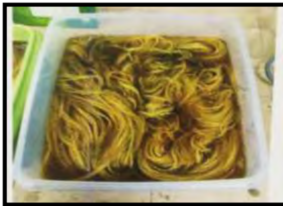
Figure 3.5: PALFs were immersed in NaOH solution
