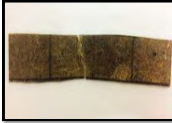
Figure 3.26: PALF/PP composite samples ruptured after tensile test
