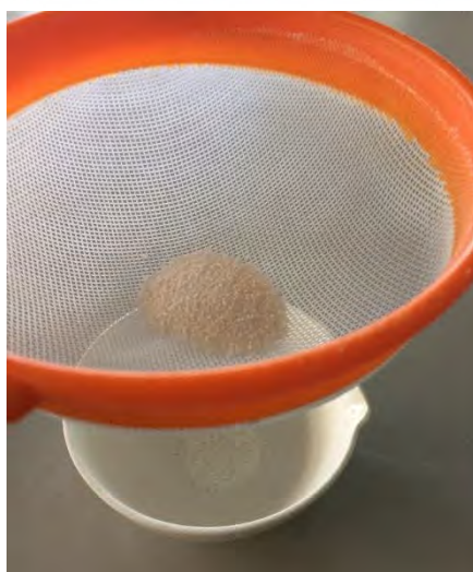
Figure 4.2 Separating fine and course sago powder
