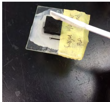
Figure 3.9 Applying 2 tons epoxy
