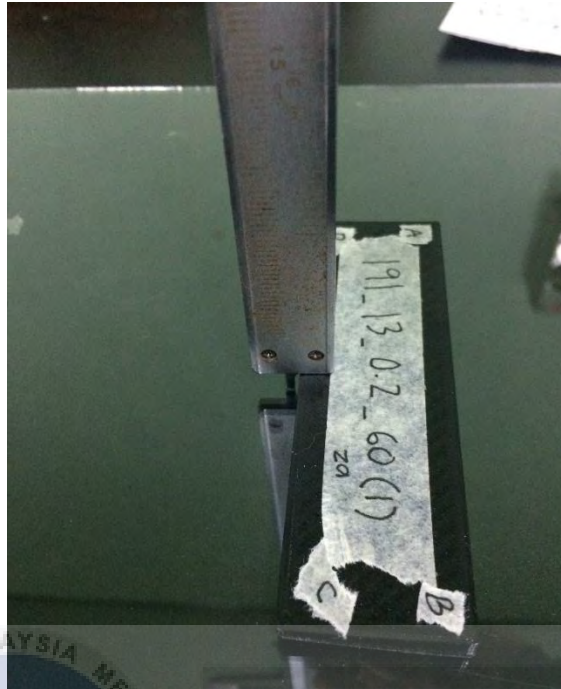
Figure 4.6(b) Measuring depth using vernier caliper
