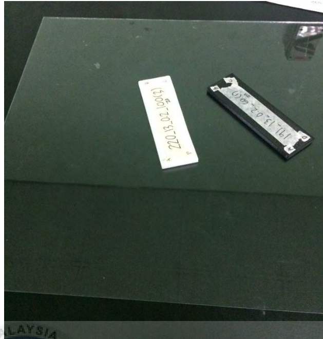
Figure 4.5 Flat glass for warping deformation measurement
