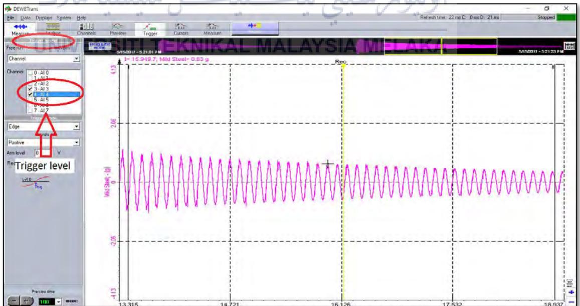
Figure 3.11: Trigger source.
