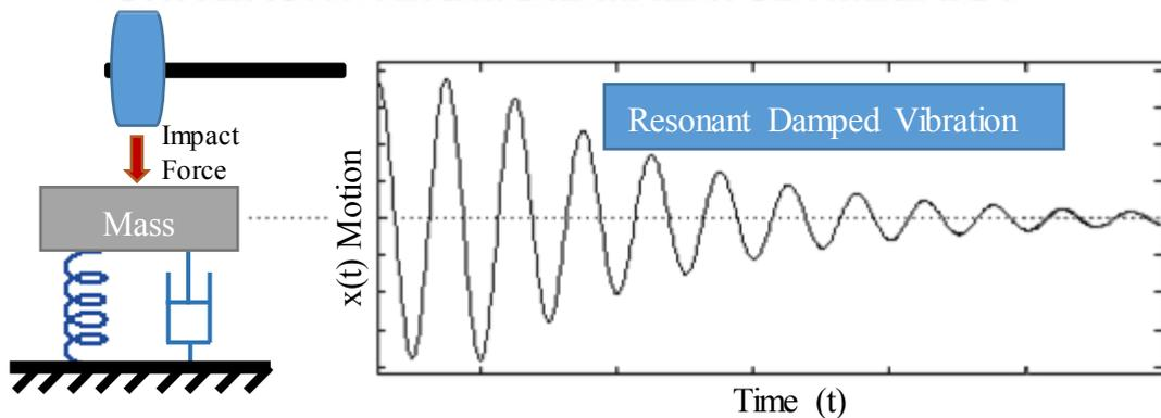
Figure 2.8: Diagram of damping propagation after an impact apply.
