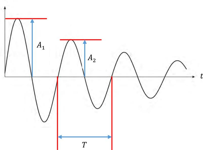
Figure 2.6: The measurement taken in logarithmic decrement.
