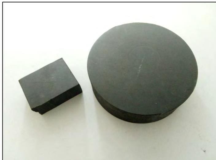
Figure 1.1: Laminated Rubber – Metal Spring (LR-MS).
