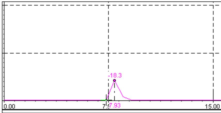
Figure 3.20: (FFT) graph signal, shows that most of the power is at one frequency after (-3dB) for Q factor calculation.
