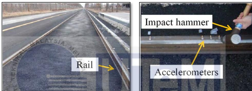
Figure 2.5: Infinitely long embedded rail and apparatus setup
