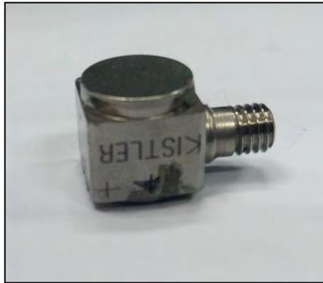
Figure 3.3: Used accelerometer device.
