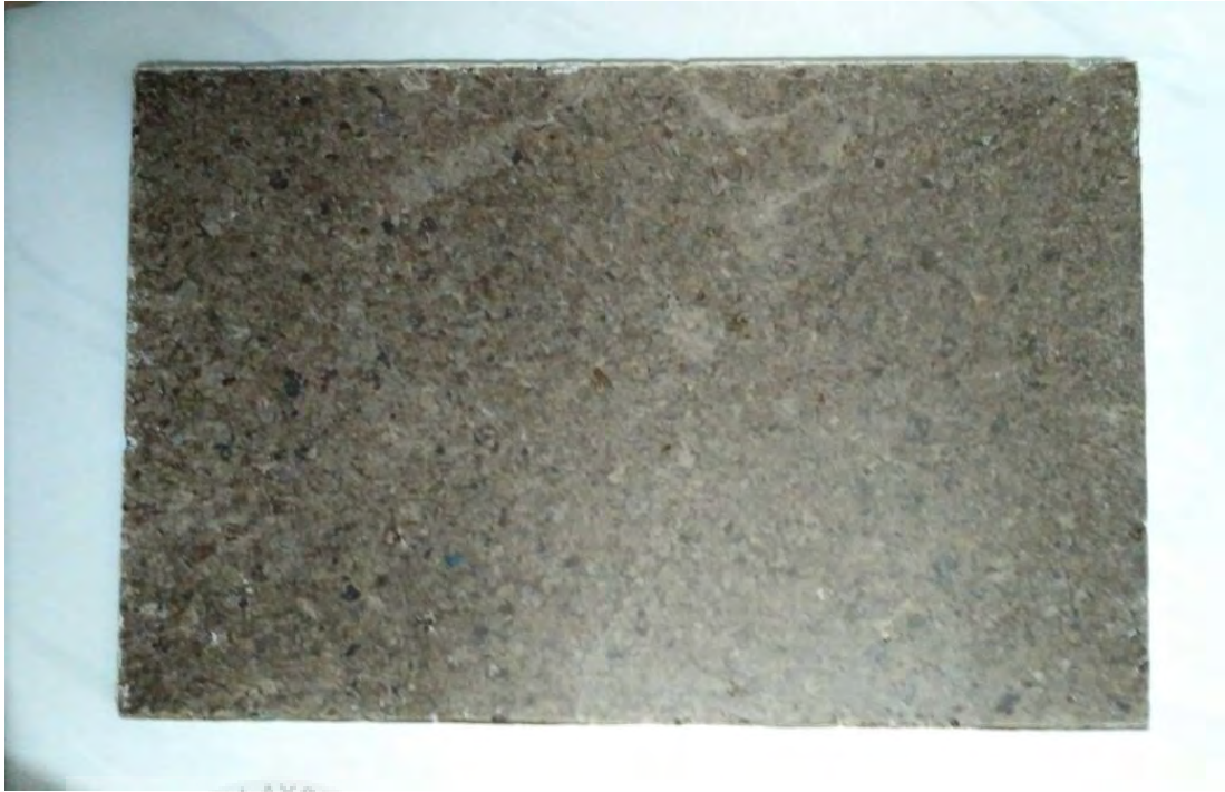
Figure 4.2-c: 20 (wt.%) kenaf to 80 (wt.%) PP specimen
