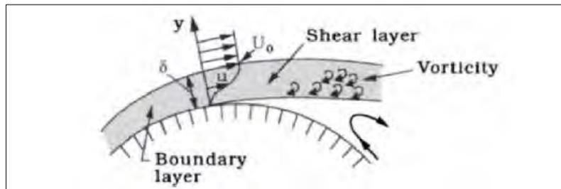
Figure 2.1: Detailed Sketch Of Flow Near Separation (Hansen et al., 2015)
