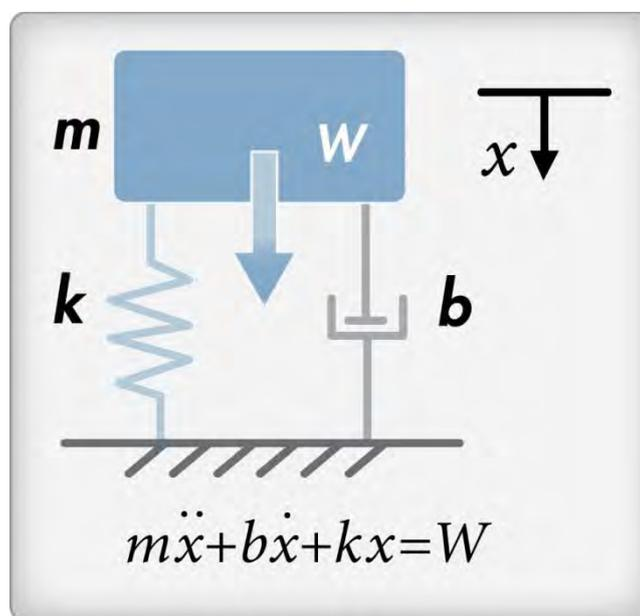
Figure 2.4 Mass-Spring-Damper System
