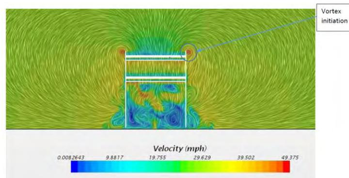
Figure 2.3 Vortex Generation From End Plates (Meederira, 2014)
