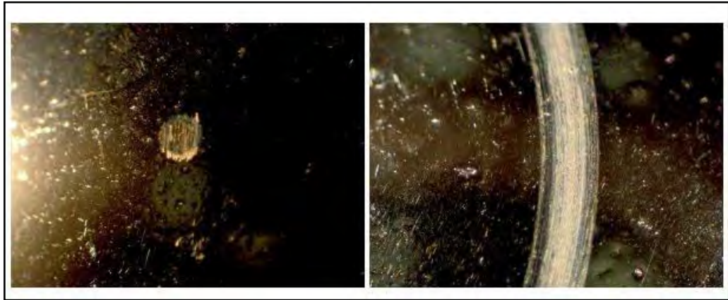
Figure 2.8: Bottom (left) and top (right) ball bearing from low-wear test using engine oil. (Les Girard, Naomi Kibrya, 2015)
