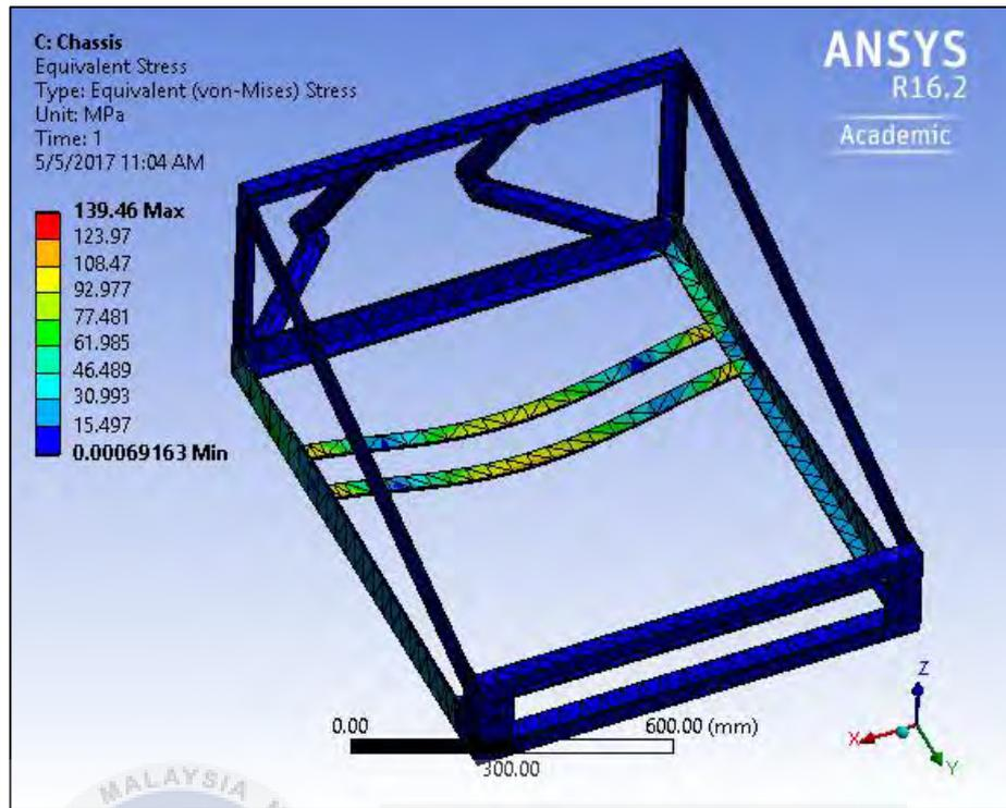
**Figure 4.28:** Von-Mises stress of aluminium alloy chassis for acceleration analysis.
