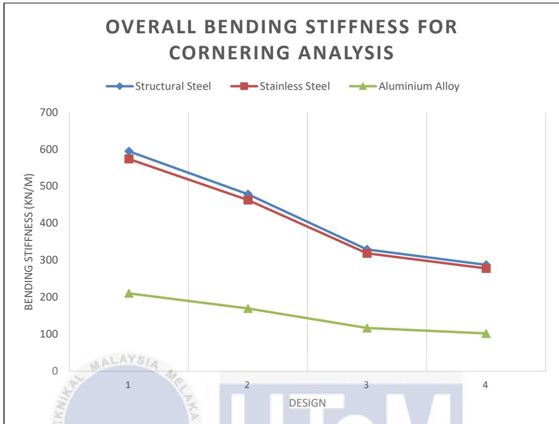
**Figure 4.13:** Bending stiffness for cornering analysis.
