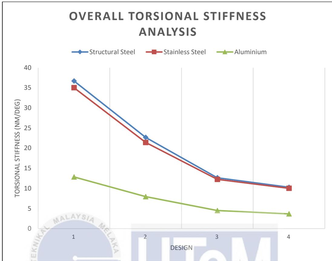
**Figure 4.16:** Overall torsional stiffness analysis.
