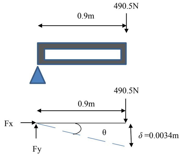
**Figure 4.15:** Free body diagram of the chassis structure with respect to frontal view.
