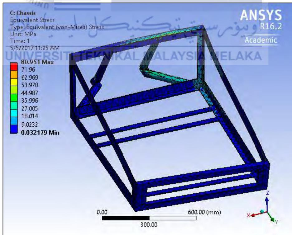
Figure 4.32: Von-mises stress of stainless steel chassis for torsional analysis.
