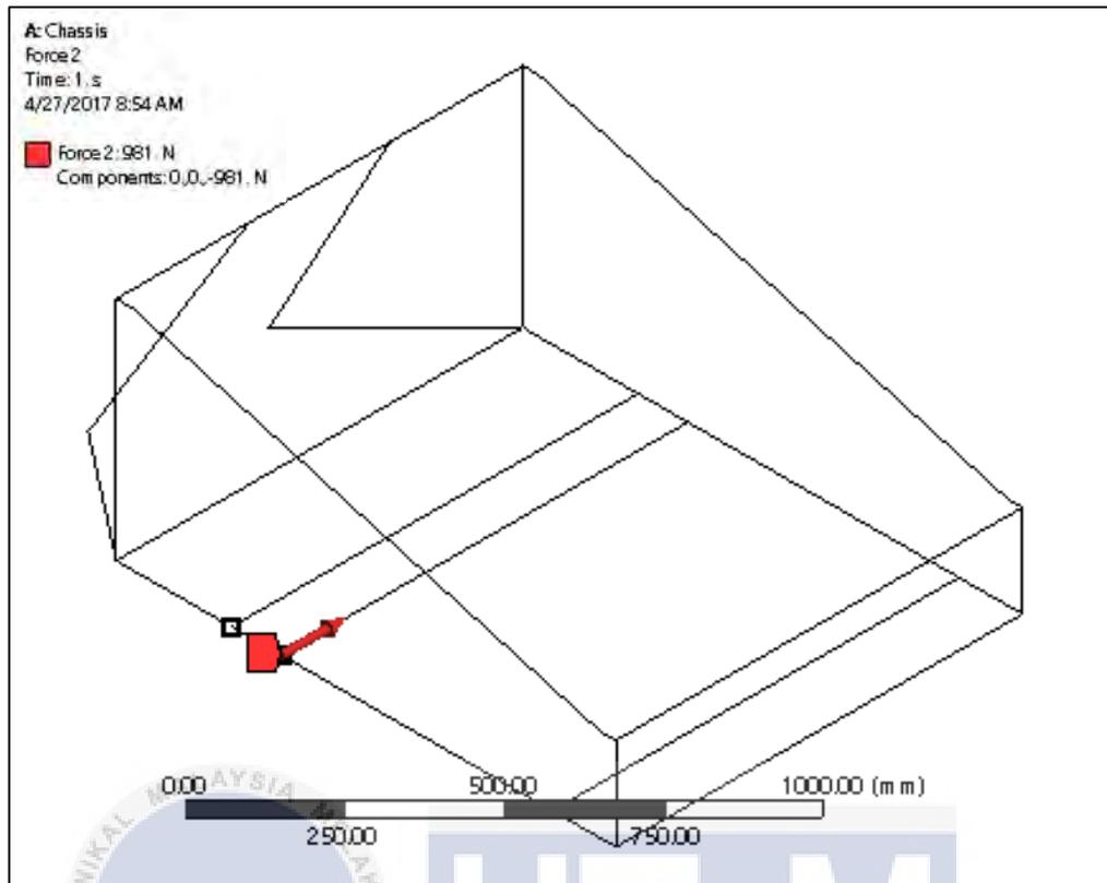
**Figure 3.16:** Computational model featuring side loads for cornering analysis.
