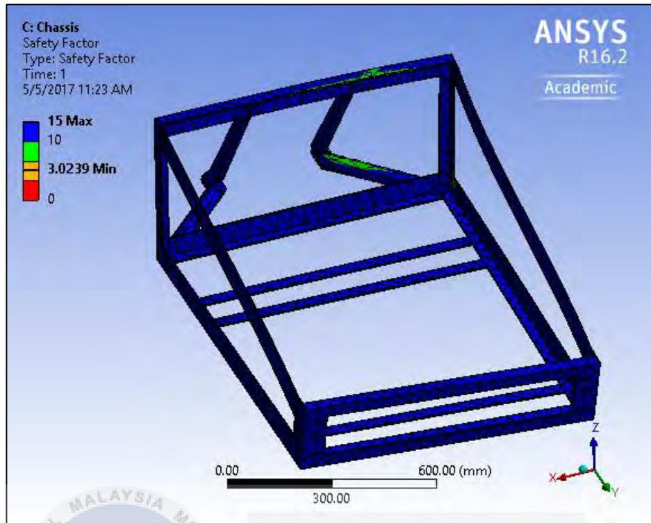
Figure 4.31: Safety factor of structural steel chassis for torsional analysis.
