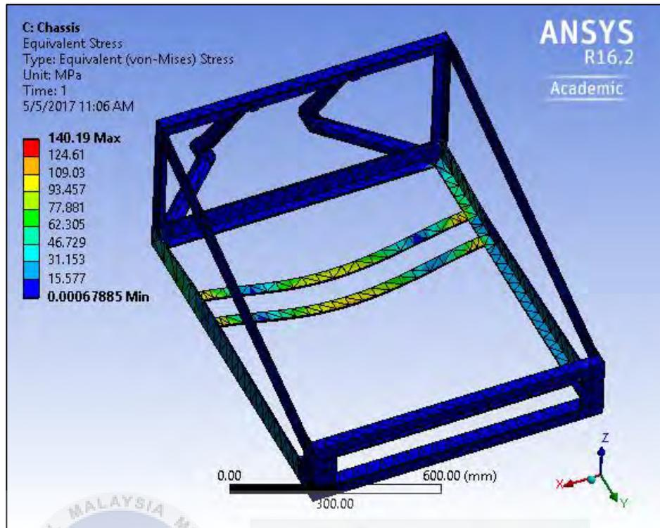
**Figure 4.24:** Von-Mises stress of structural steel chassis for acceleration analysis.
