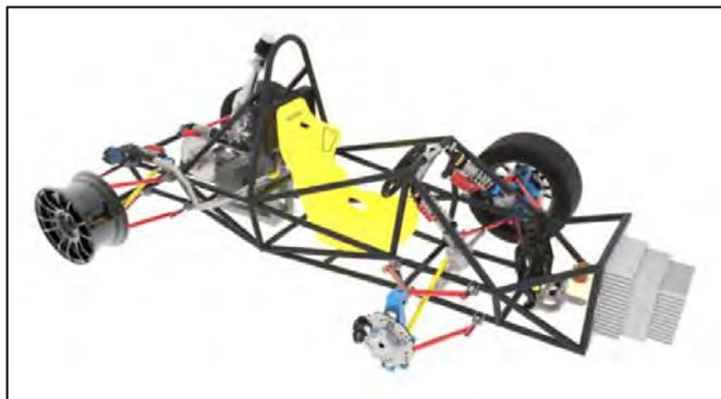
**Figure 1.1:** Frame structured in HPV (Das, 2013).
