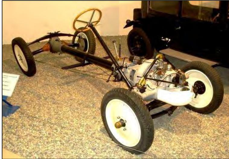
**Figure 2.4:** Model of a backbone chassis (Ludd, 2013).
