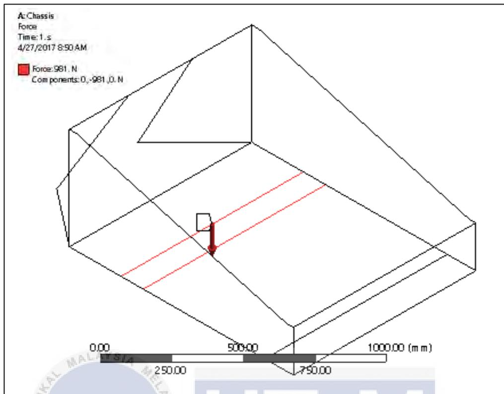
**Figure 3.14:** Computational model featuring downwards loads.
