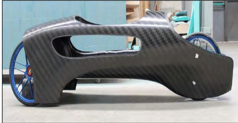
**Figure 2.6:** Model of a monocoque chassis (Carello et al., 2014).
