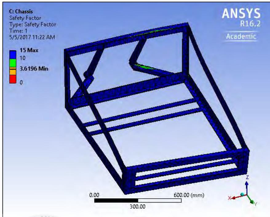
**Figure 4.35:** Safety factor of aluminum alloy chassis for torsional analysis.
