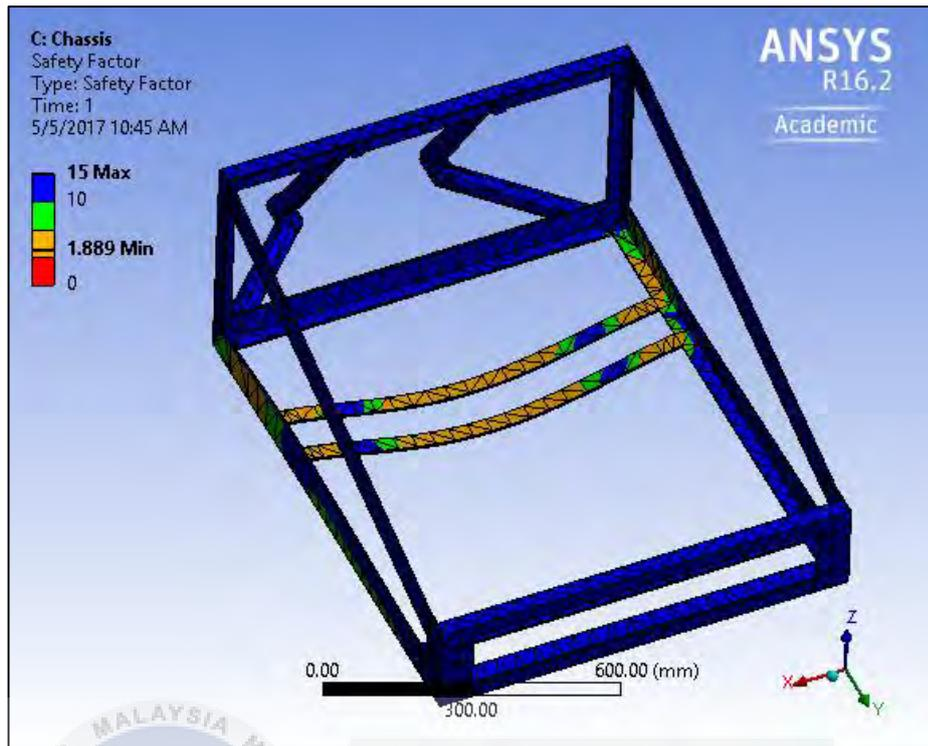
**Figure 4.19:** Safety factor of structural steel chassis for cornering analysis.
