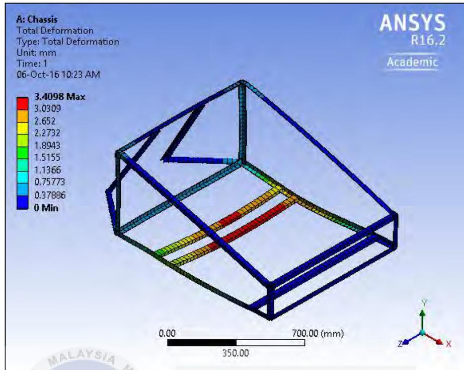
**Figure 4.2:** Fourth design of structural steel chassis for cornering analysis.
