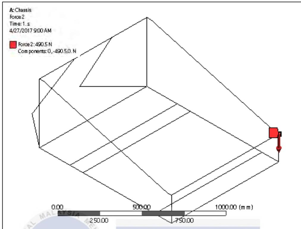
**Figure 3.12:** Computational model featuring loads for torsional analysis.
