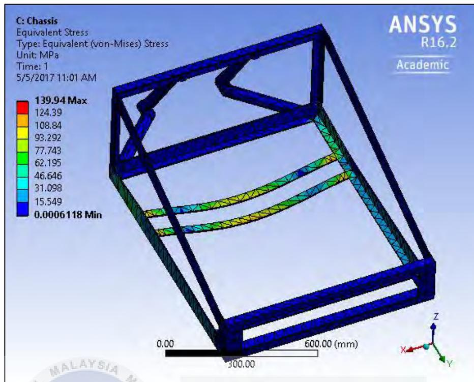
**Figure 4.26:** Von-Mises stress of stainless steel chassis for acceleration analysis.
