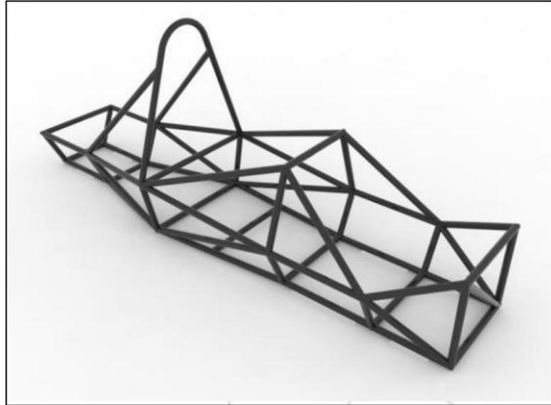
**Figure 2.5:** Model of a space frame chassis (Das, 2013).
