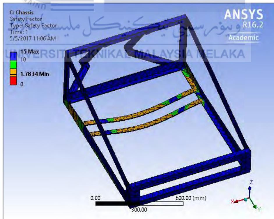
**Figure 4.25:** Safety factor of structural steel chassis for acceleration analysis.
