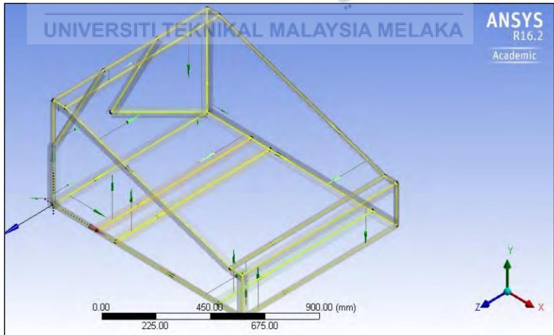
**Figure 3.6:** Model visualization with cross-sections.
