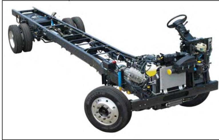
**Figure 2.3:** Model of ladder chassis (Singh et al., 2014).
