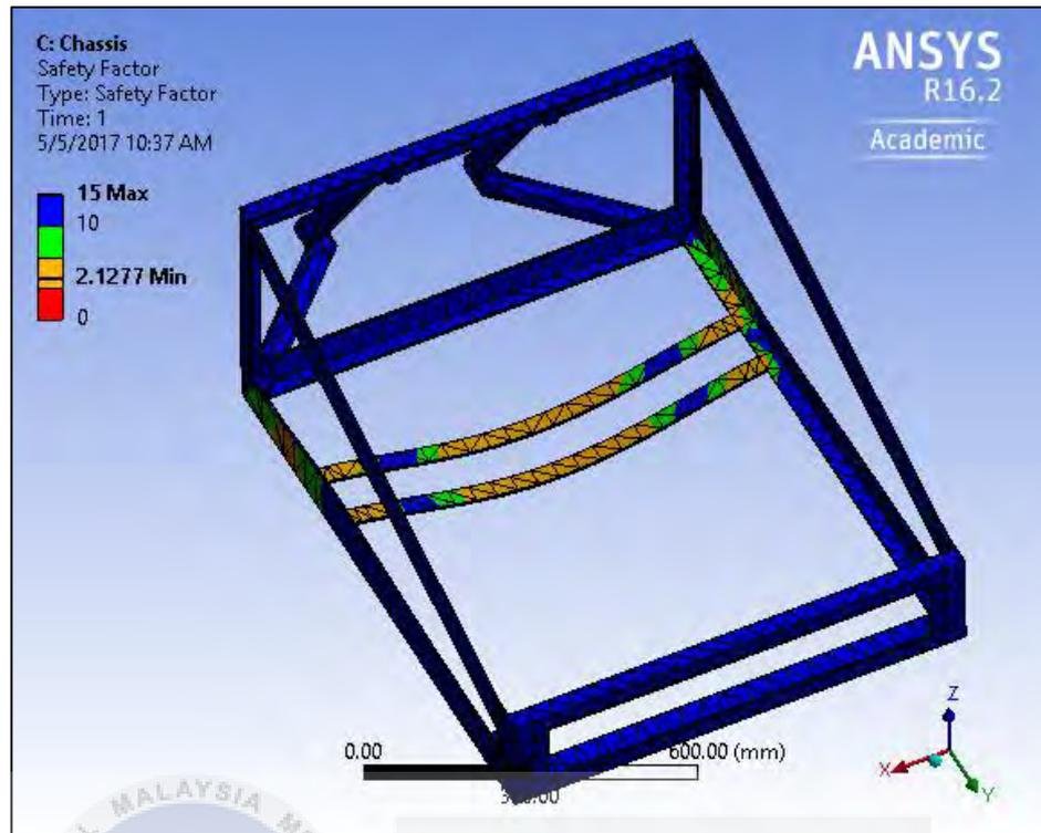
**Figure 4.23:** Safety factor of aluminium chassis for cornering analysis.
