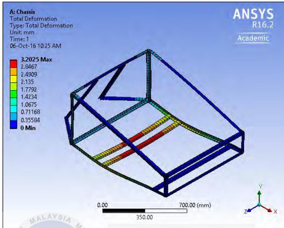
**Figure 4.6:** Fourth design of structural steel chassis for acceleration analysis.
