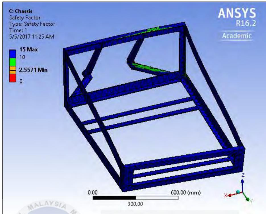
**Figure 4.33:** Safety factor of stainless steel chassis for torsional analysis.
