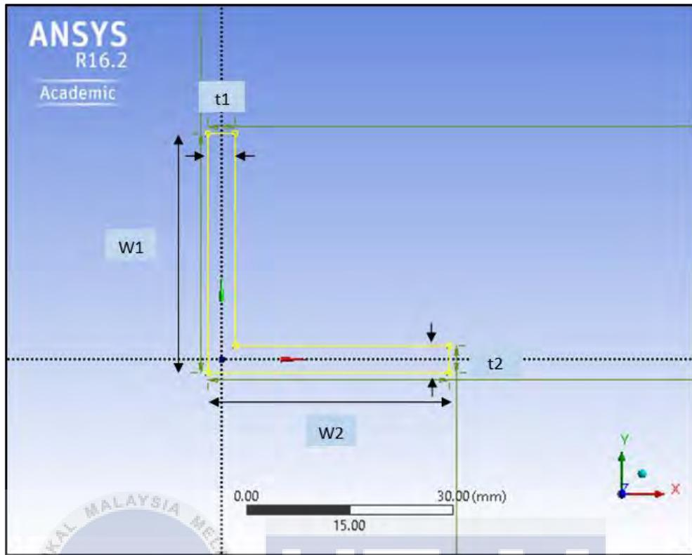
**Figure 3.7:** L-shaped cross-sectional beam.
