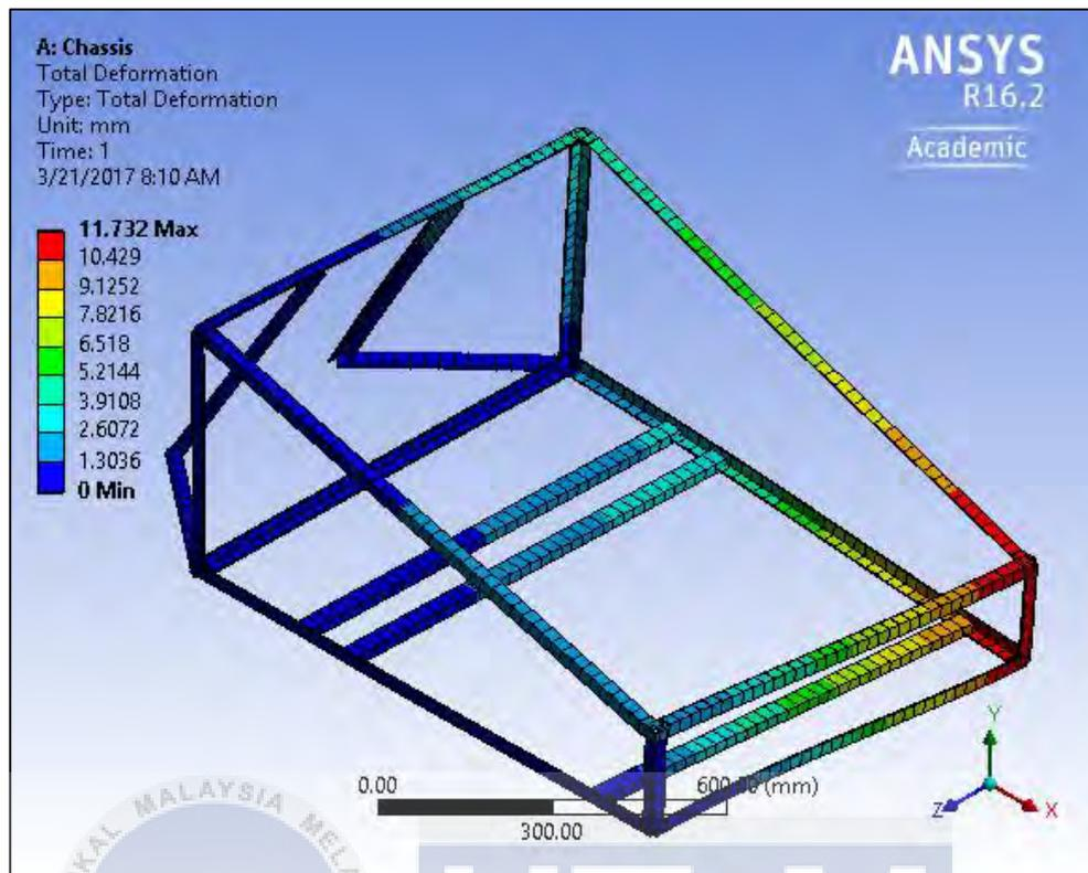
**Figure 4.10:** Fourth design of structural steel chassis for torsional analysis.
