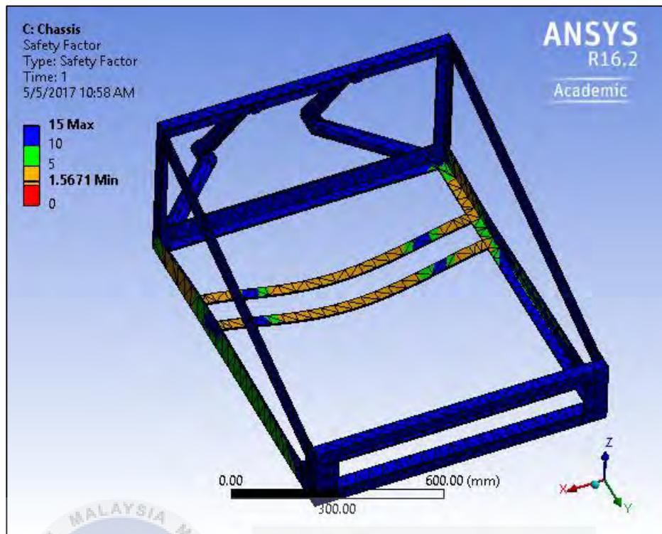
**Figure 4.21:** Safety factor of stainless steel chassis for cornering analysis.
