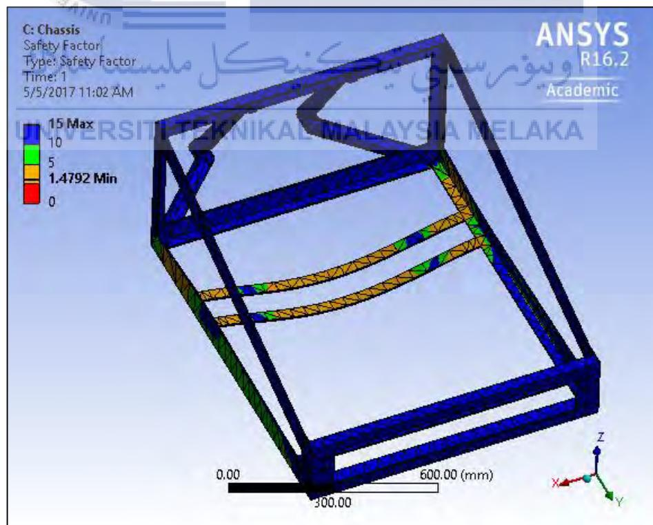
**Figure 4.27:** Safety factor of stainless steel chassis for acceleration analysis.
