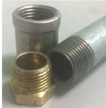
FIGURE 4.23: Extrusion system's parts with threaded ends.
