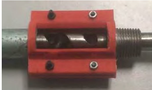
FIGURE 4.25: Installation of 3D printed clamp around the barrel.
