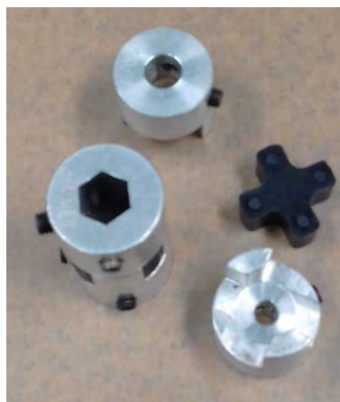
FIGURE 4.24: Spider coupling type for the shafts of the motor and drill bit.
