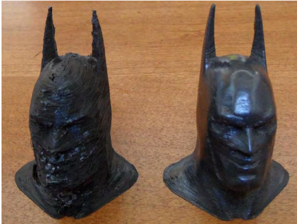
Figure 2.2: Surface finish comparison of printed parts using PLA (left) and ABS (right) ( cubex3dprinting.blogspot.my )
