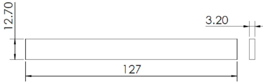
Figure 2.4(b): Specimen size for ASTM D790
