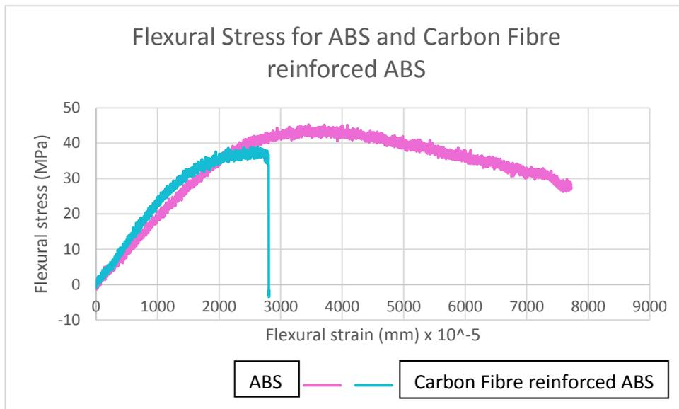
Figure 4.4: Stress-strain curves for materials ABS and Carbon Fibre reinforced ABS
