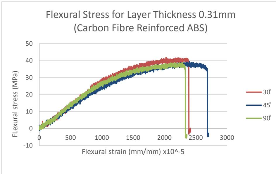
Figure 4.2(i): Stress-strain curve for flexural layer thickness 0.31mm specimens of 30°, 45° and 90° fill angle
