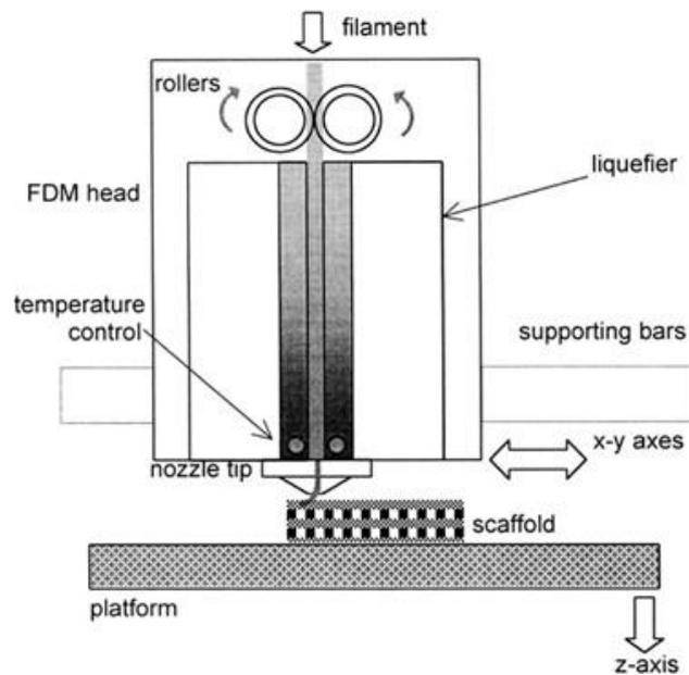
Figure 2.3(a): Schematic Diagram of 3D Printing
