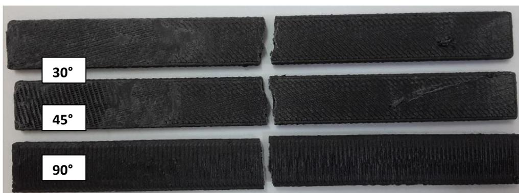
Figure 4.2(k): Fracture Flexural Carbon Fibre reinforced ABS Specimens for layer thickness 0.25mm
