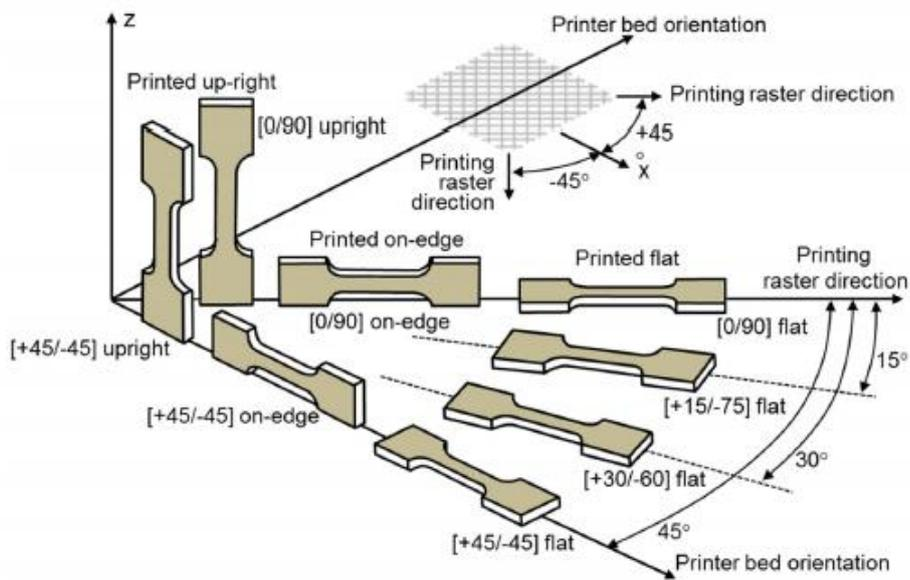
Figure 3.2(f): Illustration of the printer bed fill angles for 30°, 45° and 90°
