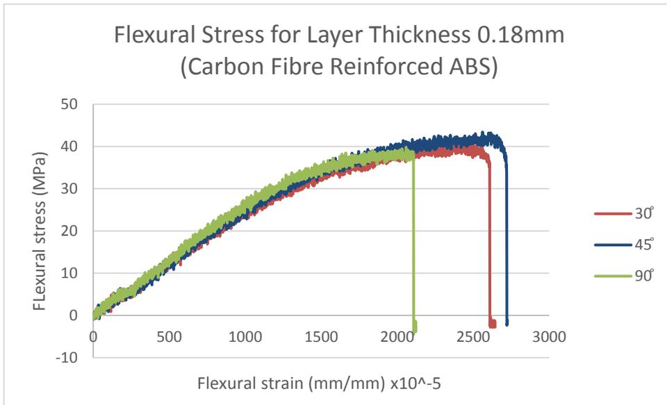
Figure 4.2(g): Stress-strain curve for flexural layer thickness 0.18mm specimens of 30°, 45° and 90° fill angle
