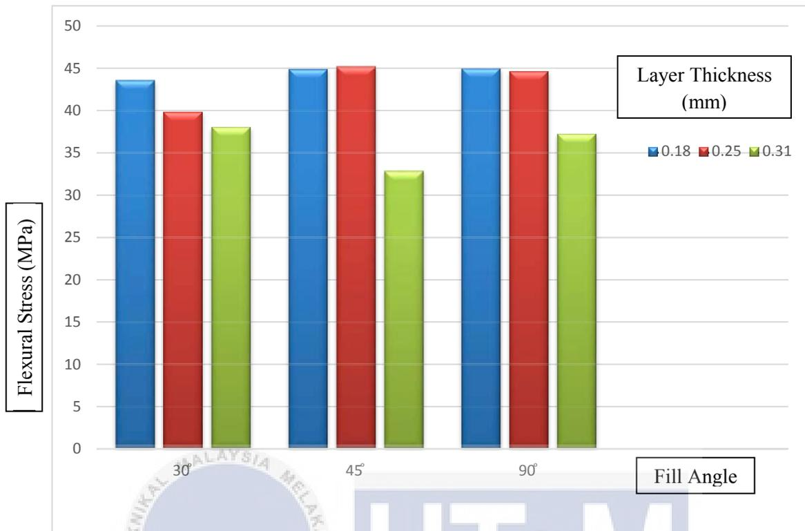
Figure 4.3(d): Bar chart for flexural fill angles for ABS material
