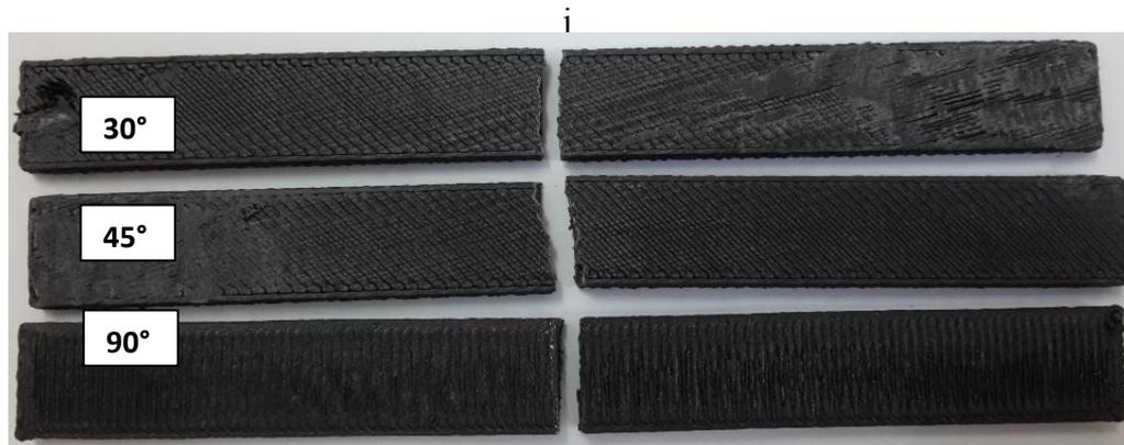
Figure 4.2(l): Fracture Flexural Carbon Fibre reinforced ABS Specimens for layer thickness 0.31mm
