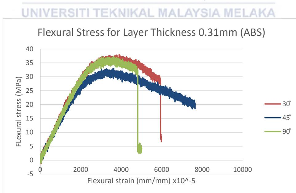
Figure 4.2(c): Stress-strain curve for flexural layer thickness 0.31mm specimens of 30°, 45° and 90° fill angle
