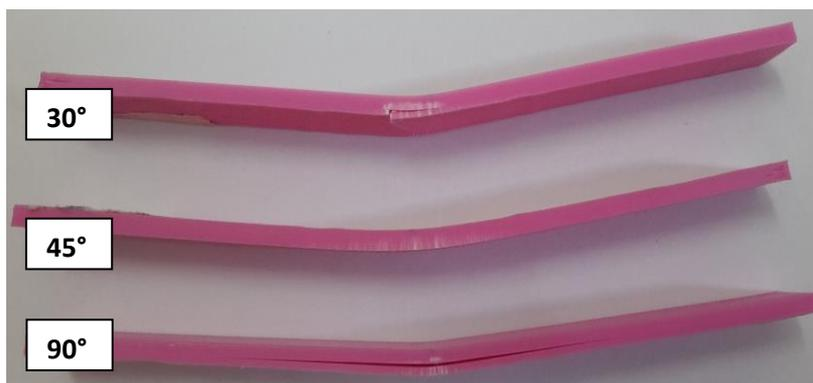
Figure 4.2(f): Fracture Flexural ABS Specimens for layer thickness 0.31mm
