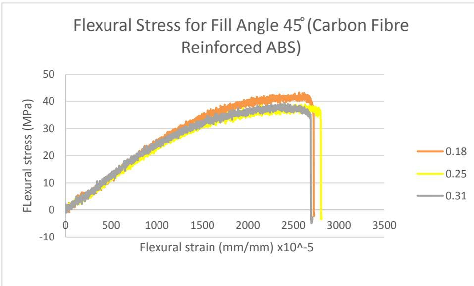
Figure 4.3(f): Stress-strain curve for flexural fill angle 45° specimens of 0.18mm, 0.25mm and 0.31mm layer thickness
