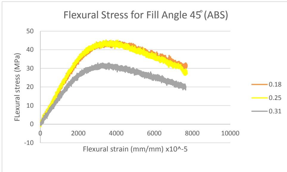
Figure 4.3(b): Stress-strain curve for flexural fill angle 45° specimens of 0.18mm, 0.25mm and 0.31mm layer thickness
