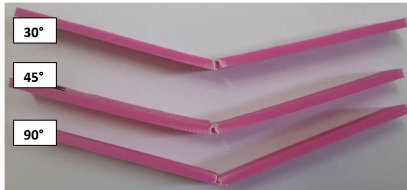
Figure 4.2(d): Fracture Flexural ABS Specimens for layer thickness 0.18mm
