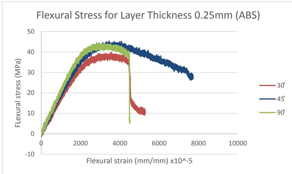
Figure 4.2(b): Stress-strain curve for flexural layer thickness 0.25mm specimens of 30°, 45° and 90° fill angle
