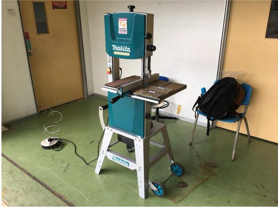
Figure 3-8 : Vertical Bench Saw
