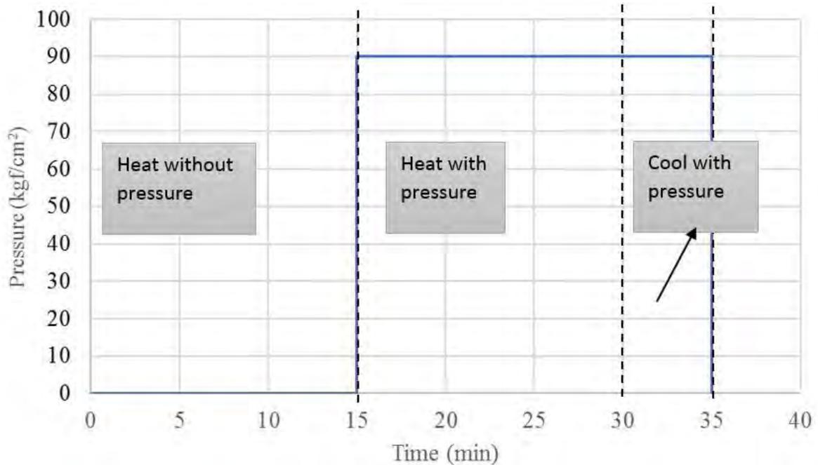
Figure 3-2 : Hot Press Process
