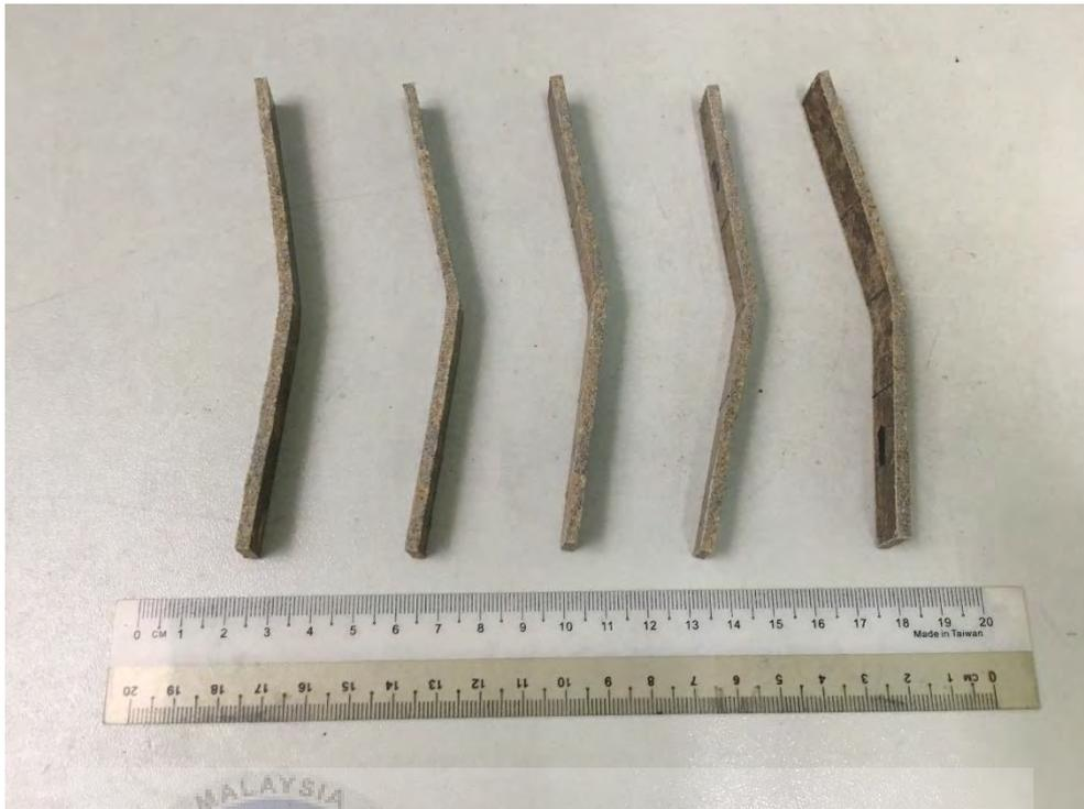
Figure 3-14: Test Samples with Composition of 10wt% OPEFB + 30wt% Kenaf + 60wt% HDPE
