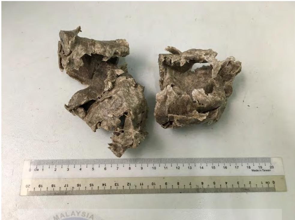
Figure 3-3 : Example of Internal Mixer Product, 40wt% Kenaf + 60wt% HDPE
