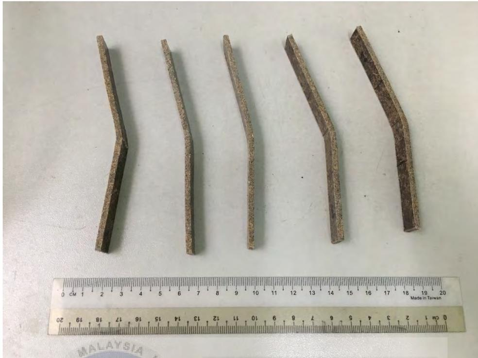
Figure 3-12 : Test Samples with Composition of 30wt% OPEFB + 10wt% Kenaf + 60wt% HDPE
