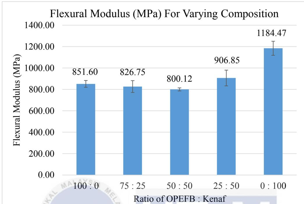
Figure 4-6 : Graph Of Flexural Modulus (MPa) For Varying Composition
