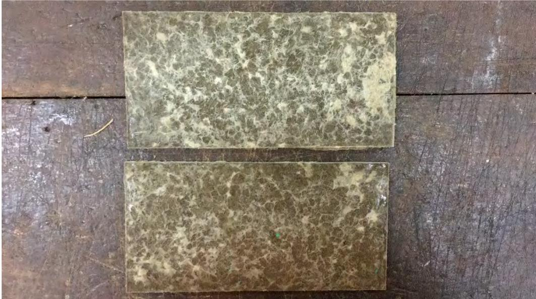
Figure 3-7 : Composite Plate Obtained After Hydraulic Hot Molding with Mold Size 200 mm x 100mm x 3.2mm
