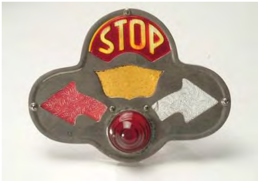
Figure 2.2: Oscar J. Simler's handmade turn signal
