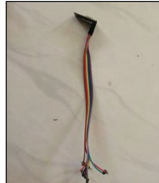
Install connecting wires to NRF24L01
