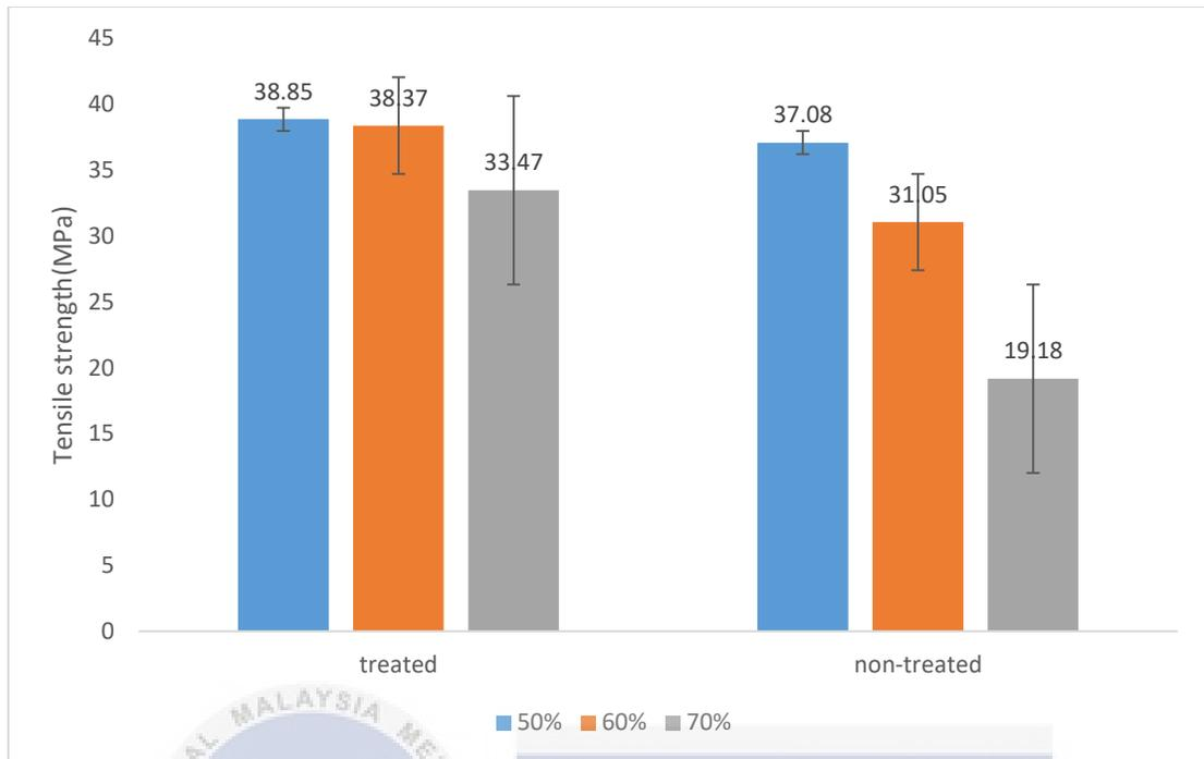
Figure 4.7: Bar graph of tensile strength of treatment and non-treatment of 90mm fibre length.
