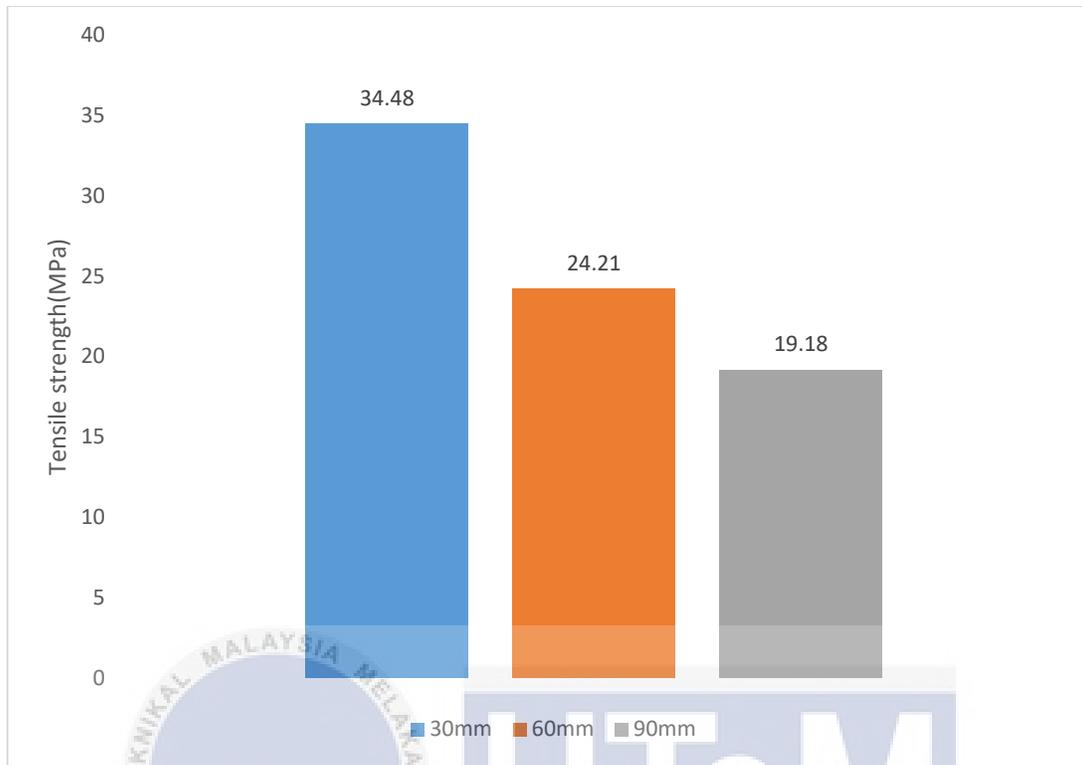
Figure 4.3: Ultimate tensile strength of FML with 70wt% and different fibre length.
