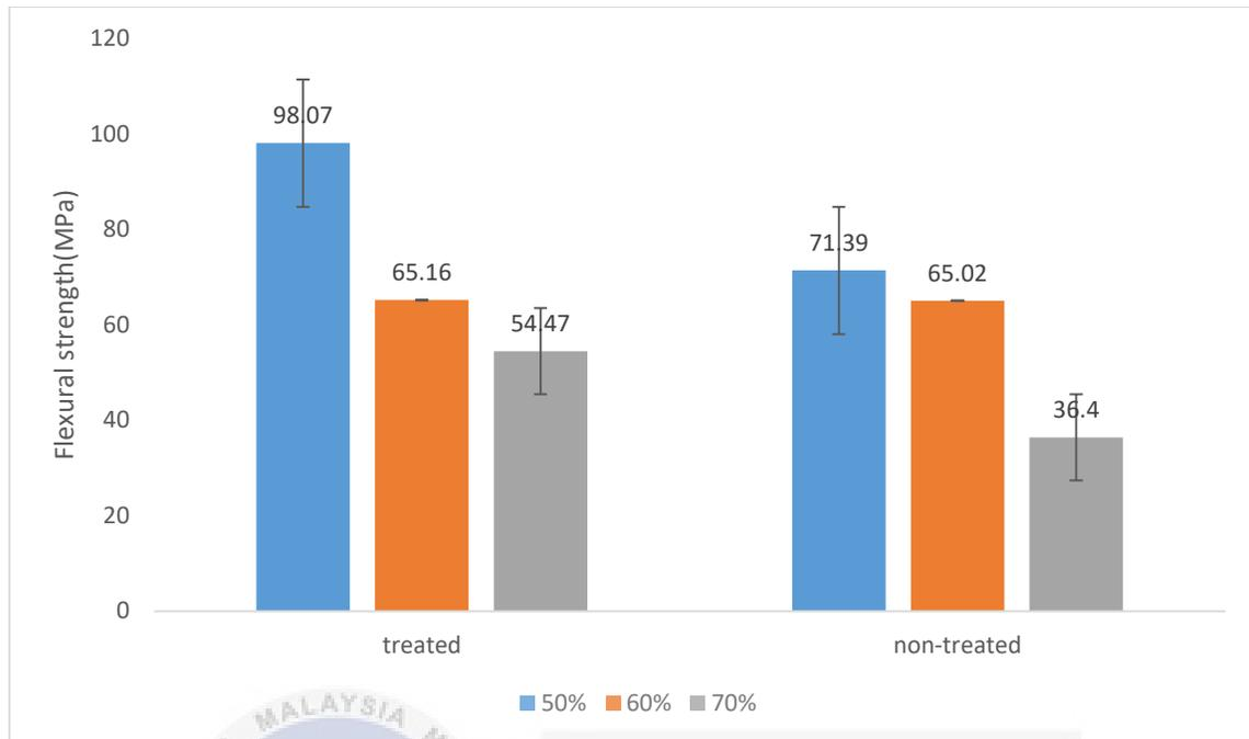
Figure 4.13: Bar graph of flexural strength of treatment and non-treatment of 60mm fibre length.
