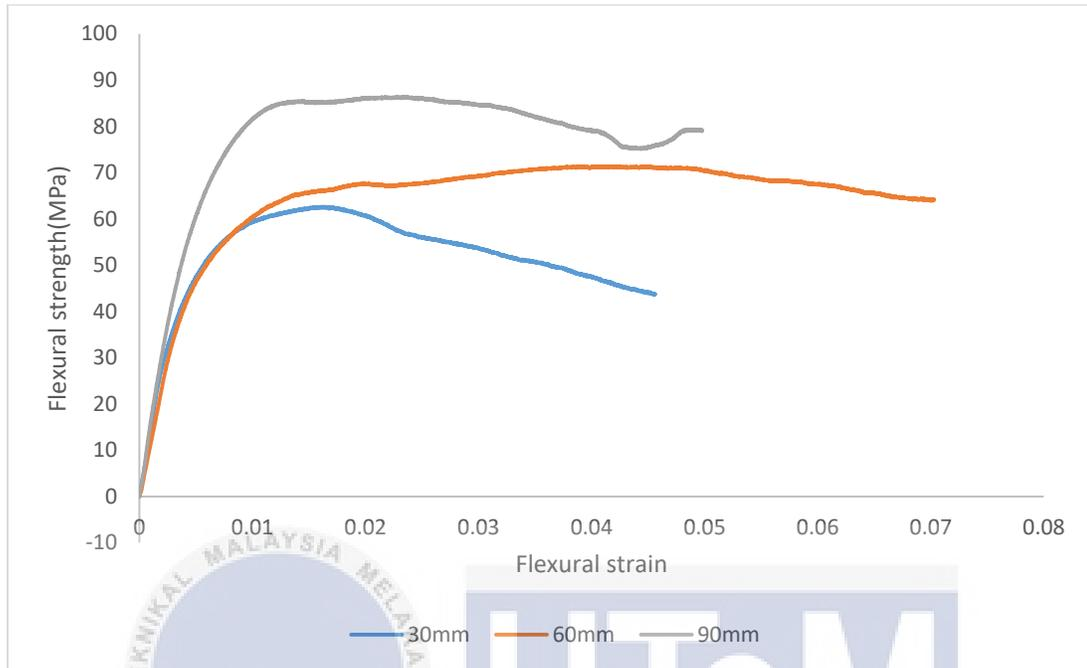
Appendix B1: Flexural stress-strain curves of FML with 50wt% and different fibre length.
