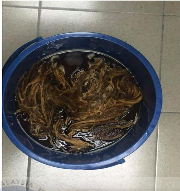
Figure 3.2: Fibre treatment in NaOH
