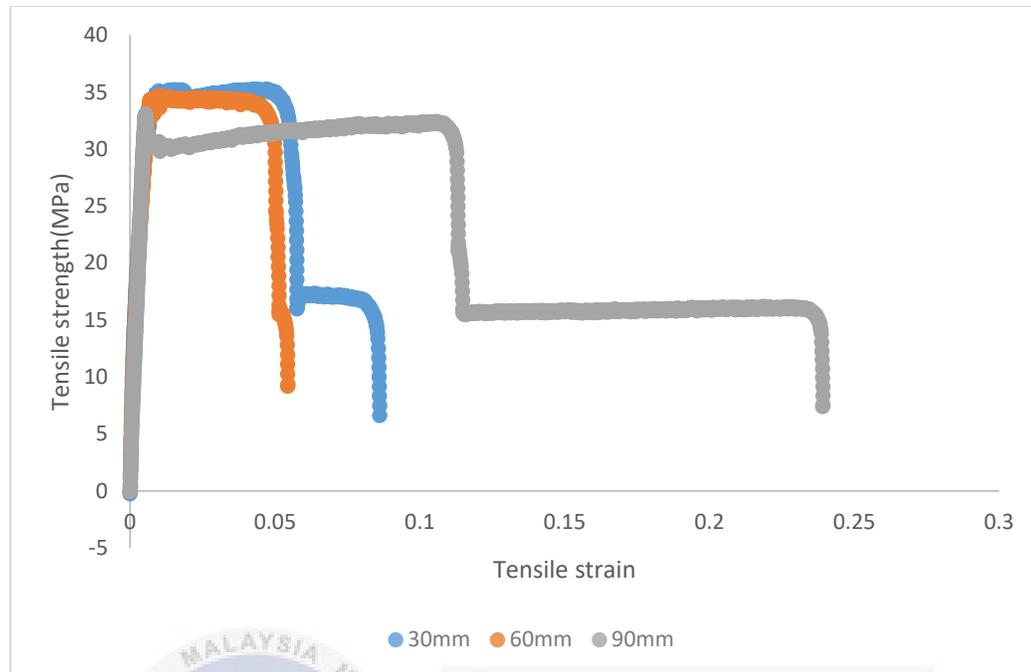
Appendix A2: Stress-strain curves of FML with 60wt% and different fibre length.
