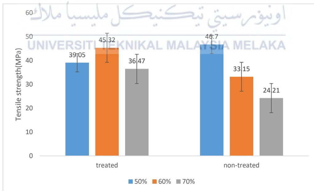
Figure 4.6: Bar graph of tensile strength of treatment and non-treatment of 60mm fibre length.
