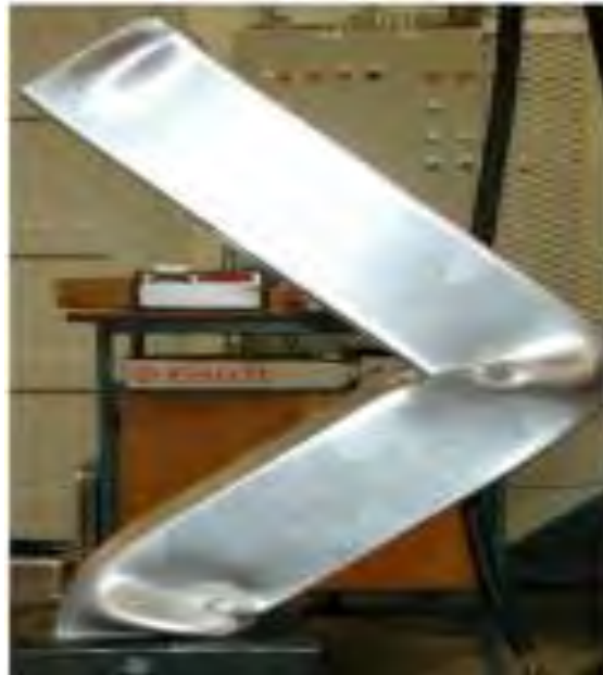
Figure 2. 6: Euler buckling deforming mode
