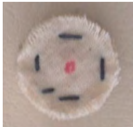
Figure 2.10: Luffa fiber with a perforated linen (Koruk and Genc, 2015)
