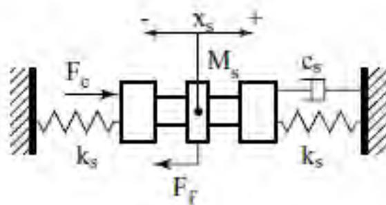
Figure 3.3: Dynamic equation of Spool valve
