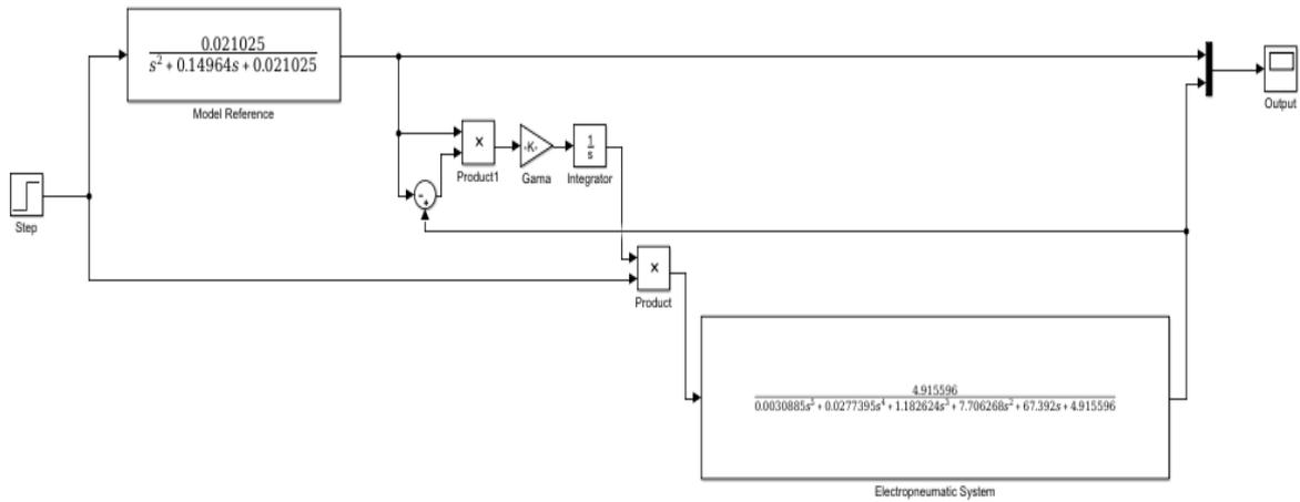
Figure 4.20: Simulink diagram of Model Reference Adaptive Control with MIT rule
