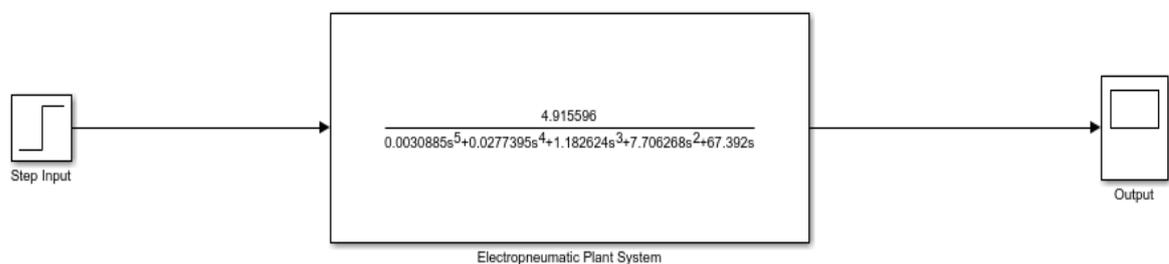
Figure 4.1: The block diagram for open loop system of electro-pneumatic plant
