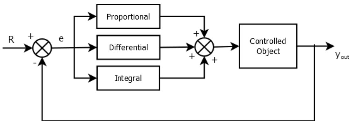
Figure 3.6: Categories of PID controller on the closed loop in control system
