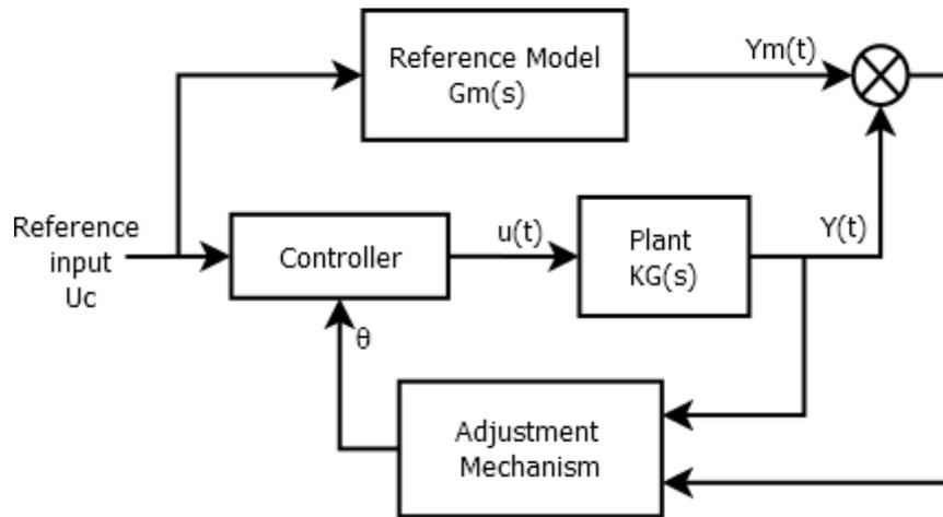
Figure 3.8: Block diagram of MRAC system
