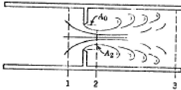
Figure 3.4: Turbulent flow through an orifice
