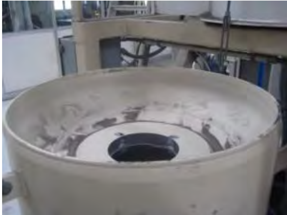
Figure 1.1: Damaged vessel wall due to damaged sealing mechanism.
