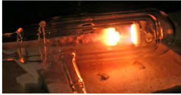
Figure 1-1 Micro combustor (micro thruster) (Fan et al, 2012)
