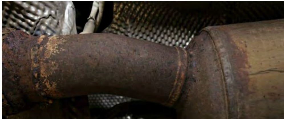
Figure 2.1: Rust and Corrosion on Joint of Exhaust Pipe
