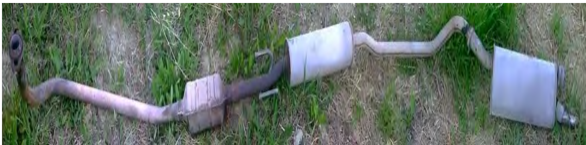
Figure 2.2: Exhaust system of the Opel Corsa B 1.2 petrol
