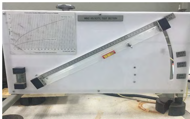
Figure 3.6.3 Slope lever of pressure of water to determine the velocity of the air in wind tunnel
