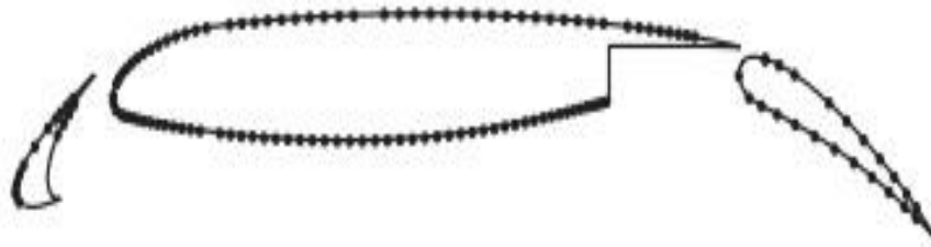
Figure 2.3.2 Schematic view of the 270 pressure tappings distributed along the airfoil chord (Pagani, Souza, & Medeiros, 2017)
