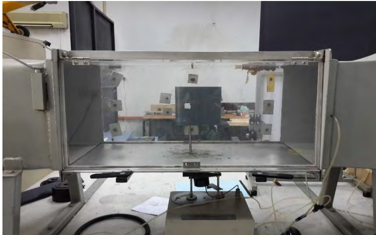
Figure 3.6.1 The middle part of the wind tunnel where subject will be tested
