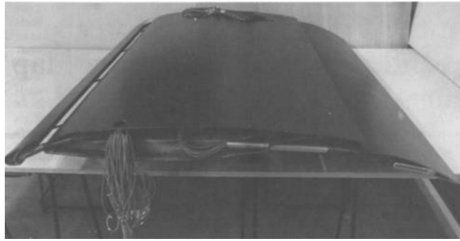
Figure 2.2.1 An A-300 series airfoil profile with leading edge slat and trailing edge flap (Savory et al., 1992)
