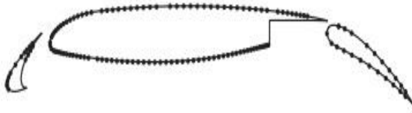
Figure 2.3.2 Schematic view of the 270 pressure tapings distributed along the airfoil chord (Pagani, Souza, & Medeiros, 2017)
