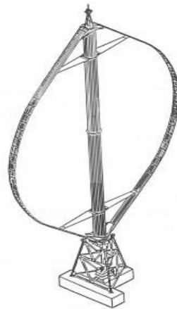
Figure 1.1 Darrieus Wind Turbine. (Source: McAdam, 2016)
