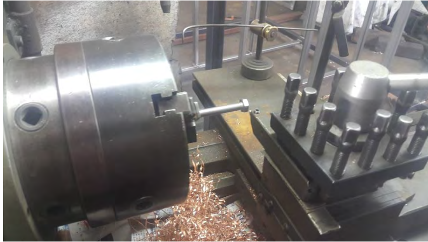
Figure 26 Conventional Lathe Machine used in the process of fabricating the shaft
