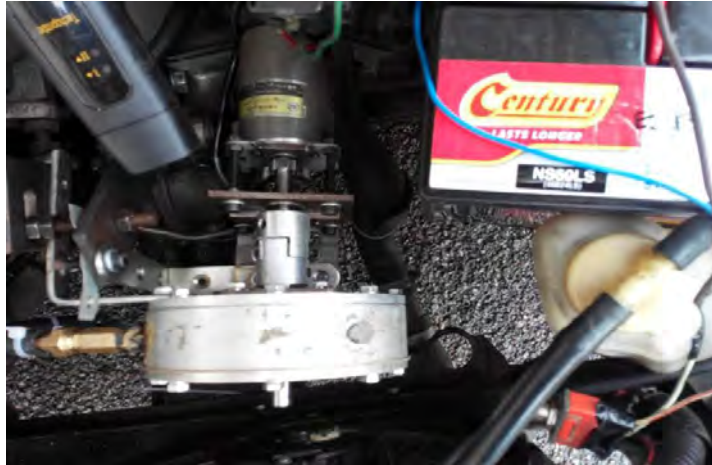
Figure 10 The position of the generator under the car hood (Herawan et al., 2015)
