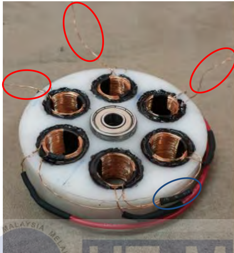
Figure 24 shows the life and neutral output of generator
