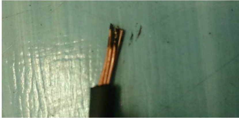
Figure 4.14: Wire burnt as too hot and connecting with the clip holder.
