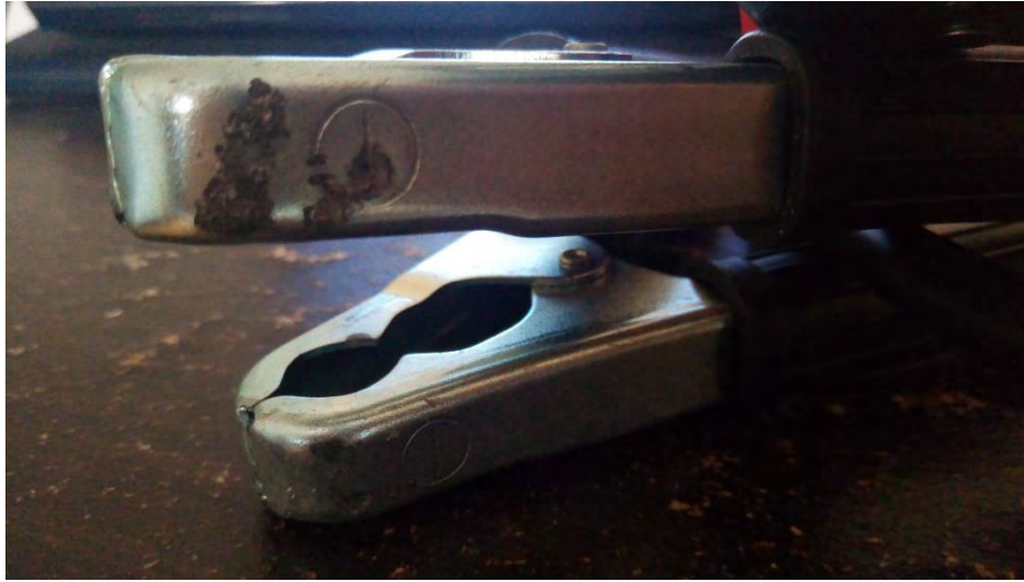
Figure 4.15: Implication of spark and short circuit to clip holder.
