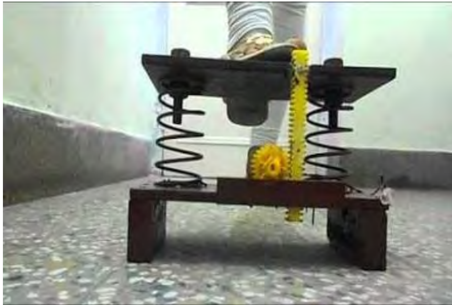
Figure 2.1 : Road power generation from rack and pinion system.
