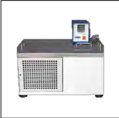
Figure 3.5: Water bath (PROTECH, 2008).
