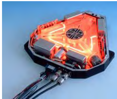
Figure 2. 2: Example of Ring Laser Gyroscope (RLG)
