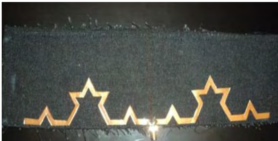
Figure 1.2: Fabricated Koch Fractal dipole antenna (Pratik Patel et al., 2013)
