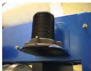
Figure 2.14: The Pressure sensor as depth sensor [19]
