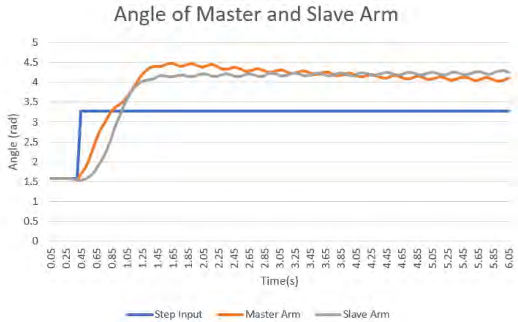
Figure 4.14: Angle of from master and slave arm rotated from its original position with value of K_p=20 and K_d=1.6 .
