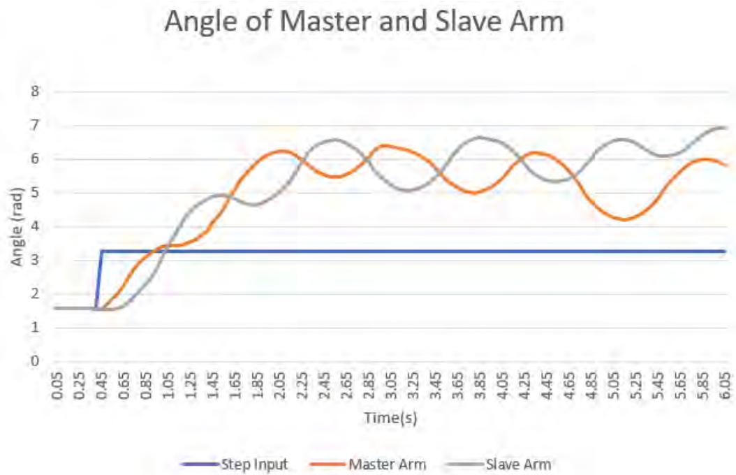
Figure 4.8: Angle of from master and slave arm rotated from its original position with value of K_p=20 .
