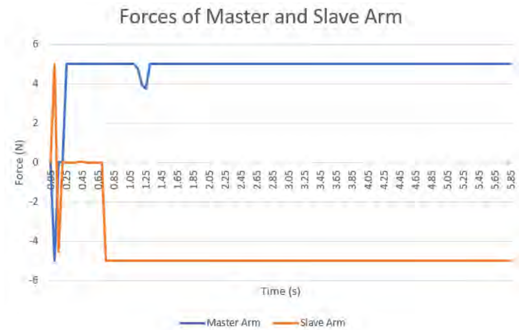
Figure 4.1: Force data from master and slave arm with the maximum torque of 5N.
