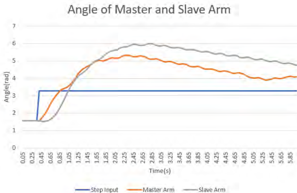
Figure 4.21: Angle of from master and slave arm rotated from its original position with value of K_p=50 , K_d=4.65 and K_i=0.05 .
