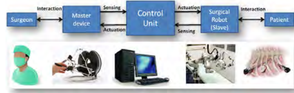
Figure 2.4: Example of closed-loop teleoperation of surgery which control unit is between master and slave arm.
