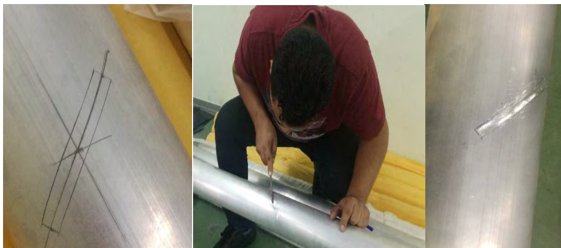
Figure 3.16: 3 mm depth oblique defect
