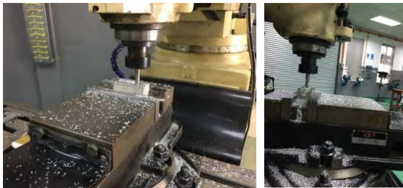
Figure 3.5: Vertical milling machine during the process during of fabrication the transducer
