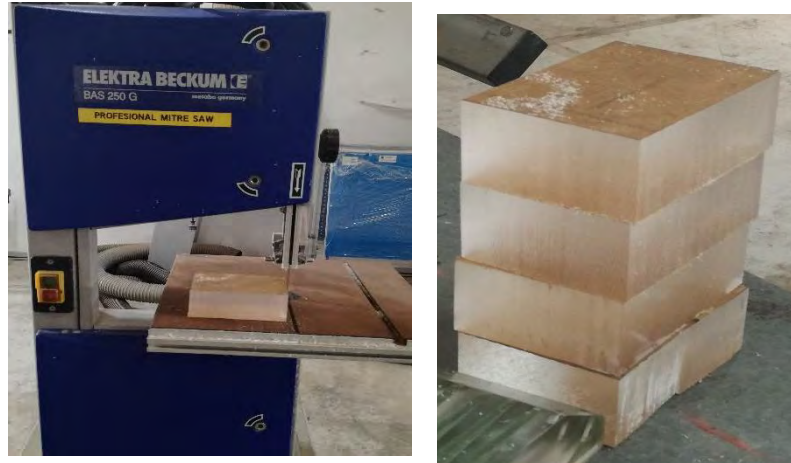
Figure 3.10: Cutting acrylic plates for transducer shoes
