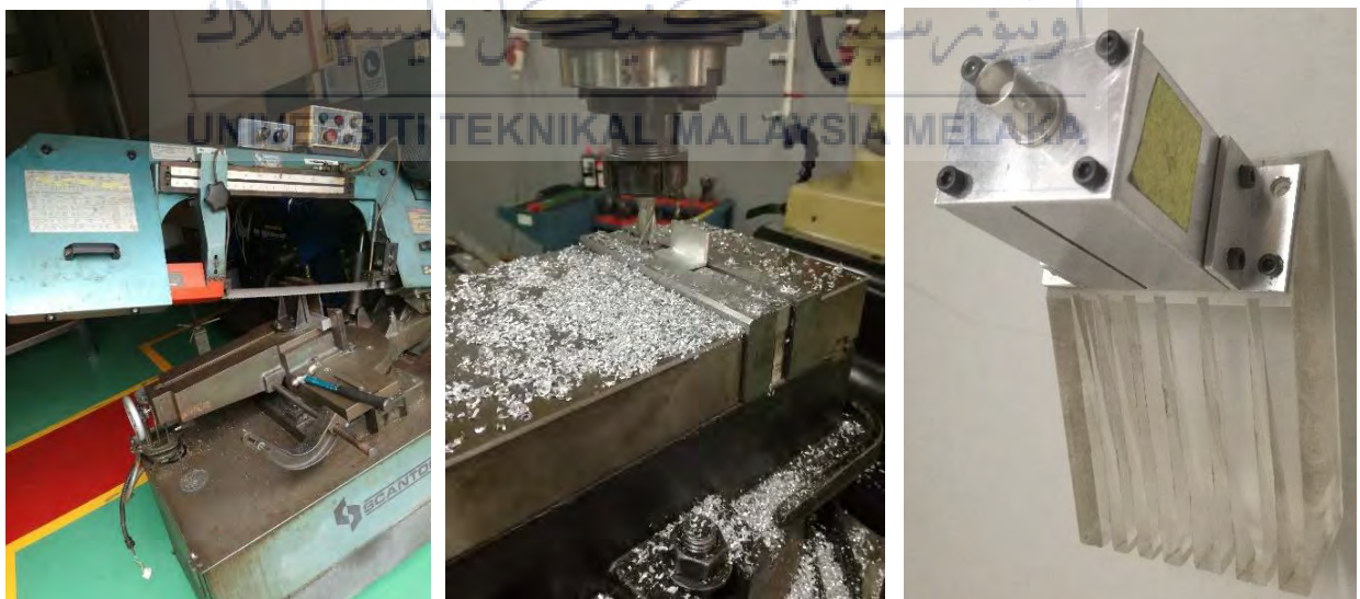
Figure 3.13: Holders fabricating processes
