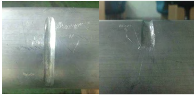
Figure 3.15: 3 mm depth defect – top view, side view
