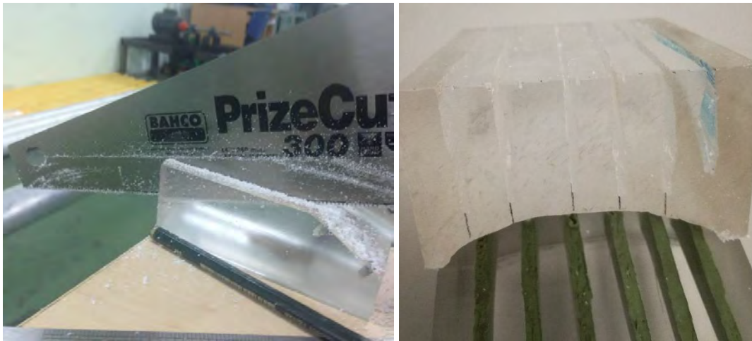
Figure 3.12: Fabricating the grooves on the acrylic shoe
